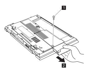
Note: The hard disk is attached to the cover.
