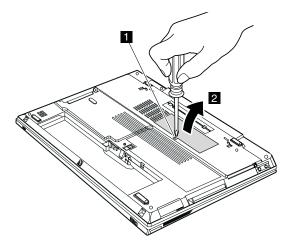
Note: Loosen the screw 1 but do not remove it.
