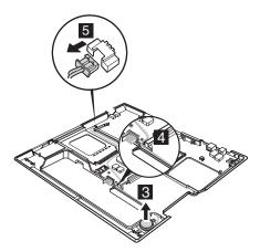
When installing: Make sure that you fasten the connector firmly.
