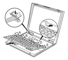
2. Align the tabs of the keyboard with the corresponding slots; then press the keyboard until it snaps into place.
