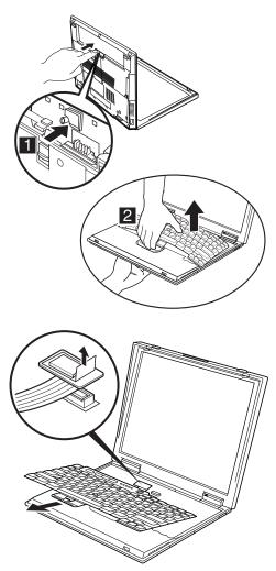
When installing: When installing the keyboard, do as follows:
