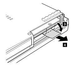
When installing: Make sure that the hard disk drive connector is attached firmly.
