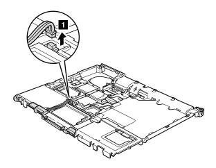
When installing: Make sure that the speaker connector is attached firmly.
