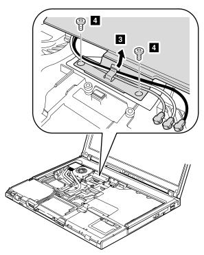
In step **3**, release the wireless antenna cables from the cable guide.
