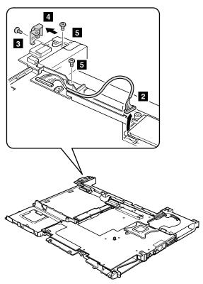
In step 4, remove the security hole bracket in the direction of the arrow.
