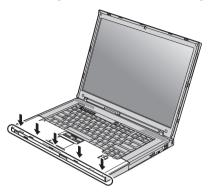
d. Close the computer display, and turn the computer over. Reinstall the four screws for the palm rest.
