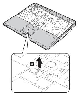
When installing: If the ThinkPad computer you are servicing has the touch pad, make sure that the connector a is firmly attached.
