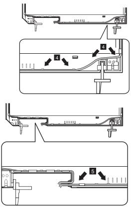
Secure the antenna assembly and hinges with screws to the LCD cover.
