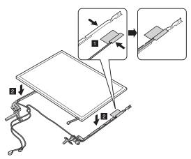
2. Place the antenna assembly on the LCD. (continued)
