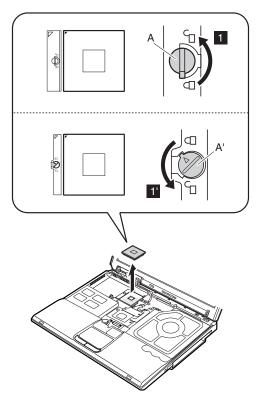
When installing: Place the CPU on the CPU socket (1), and then rotate the head of the screw (A) in the direction of arrow 2 to secure the CPU.
