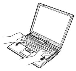
Secure the keyboard from the bottom of the computer, using the new screws provided with the keyboard.
