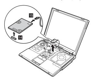
When installing: Make sure that connectors 14 and 15 are firmly attached.
