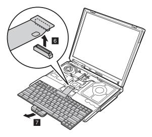
When installing: Make sure that connector 6 is firmly attached.
