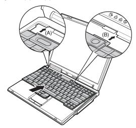
3. Press the keys indicated by arrows to latch the keyboard firmly in place.
