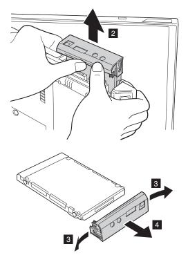
When installing: Make sure that the hard-disk connector is firmly attached.
