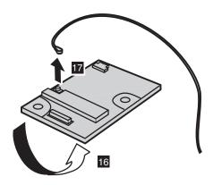
When installing: Make sure that antenna jack 17 is firmly attached.
