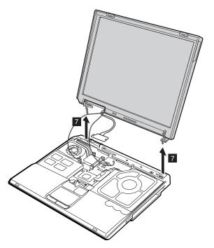
When installing: Make sure that the antenna cables are routed along the cable holder as shown in this figure, and then attach the LCD assembly to the base cover by securing the screws.
