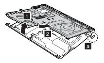
Note: To remove the system board, the lever a must be pulled out.
