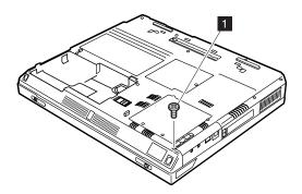
Note: The hard disk is attached to the cover.
