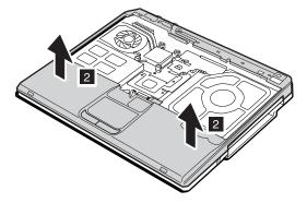
Removing and replacing a FRU
