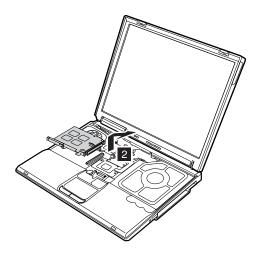
When installing: Make sure that the connector of the PC card slot is firmly attached, and then secure the screws.
