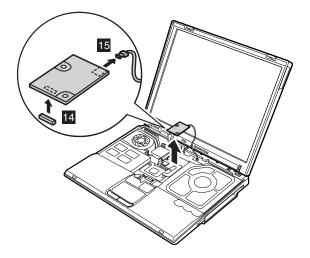
When installing: Make sure that connectors 14 and 15 are firmly attached.
