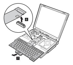
When installing: Make sure that connector **6** is firmly attached.
