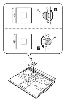
When installing: Place the CPU on the CPU socket (1), and then rotate the head of the screw (A) in the direction of arrow 2 to secure the CPU.
