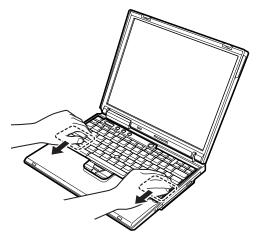
5. Secure the keyboard from the bottom of the computer, using the new screws provided with the keyboard.
