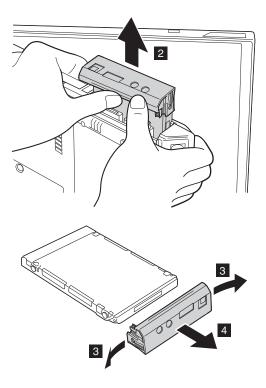
When installing: Make sure that the hard-disk connector is firmly attached.
