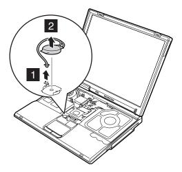
When installing: Make sure that the connector **1** is firmly attached.
