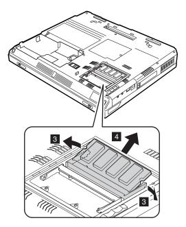
When installing: With the notched end of the DIMM toward the socket, insert the DIMM into the socket, and then press it firmly. Pivot the DIMM until it snaps into place. Make sure that the card is firmly fixed in the slot and does not move easily.
