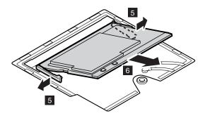
When installing: With the notched end of the card toward the socket, insert the card into the socket, and then press it firmly. Pivot the card until it snaps into place. Make sure that the card is firmly fixed in the slot and does not move easily.
