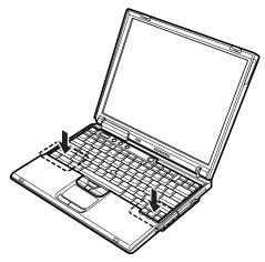
To make sure that the front side of the keyboard is housed firmly, gently press the keys with your thumbs and try to slide the keyboard towards you.
