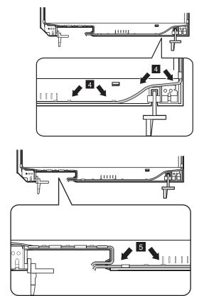
Secure the antenna assembly and hinges with screws to the LCD cover.
