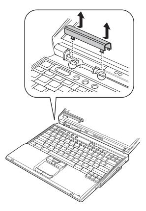
When installing: Attach the hinge cover, aligning the two projections on the rear side with the two small square holes of the base cover.
