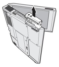
6. Do not remove the screws from the sides of the cover; instead, detach the cover from the hard disk drive by pulling in the direction of the arrows, first 1 and then 2.
