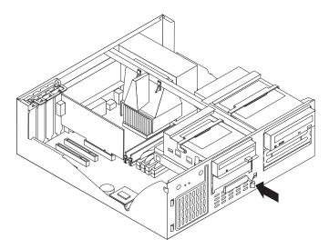
3. Swing the 3.5" drive cage up and latch into vertical.
