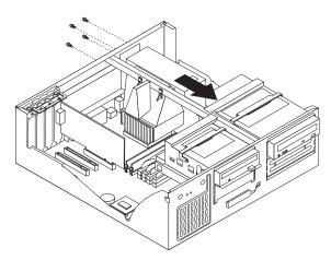
2. The power supply is attached to the base of the chassis by a latch on the front. Slide the power supply forward to dislatch if from the chassis.
