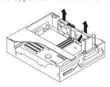
2. Press down on the tab, slide the bracket back and lift up.
