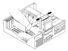
3. When replacing the drive cage into its horizontal position, be sure place the cage latch back to its regular horizontal position. This is necessary so that the machine cover will fit properly.
