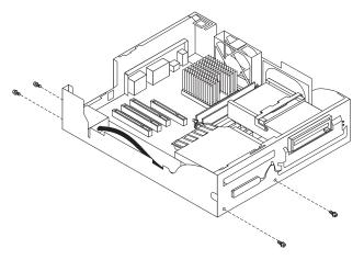
3. Locate the two tabs that secure the CD-ROM drive bracket to the back of the power supply. Push in the two tabs and remove the bracket.
