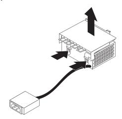
4. Lift out the power supply and plug.
