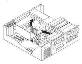
2. If the air duct does not have a hole, simply swing out the duct to a 45-degree angle and lift it up.
