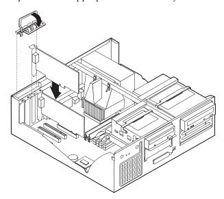
4. Install the adapter slot cover latch. Pivot the latch back to horizontal
