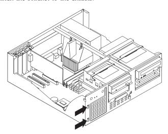
2. Locate the right tab that hinges the fan/speaker bracket to the chassis. Push the tab to detach the bracket from the chassis.
