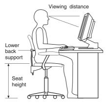
Adjust the monitor so that the top of the screen is at, or slightly below, eye level. Place the monitor at a comfortable viewing distance, usually 51 to 61 cm (20 to 24 in.), and position it so that you can view it without having to twist your body.
