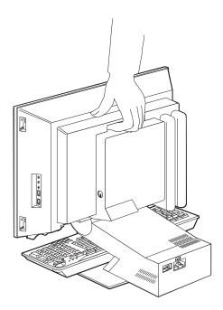
7. If you are moving your computer other than a short distance and you saved the original shipping cartons and packing materials, use them to pack the units. If you are using different cartons, cushion the units to avoid damage.
