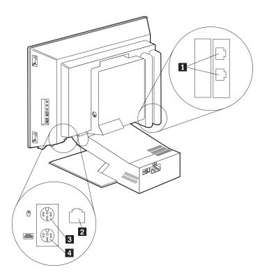
1 Modem connector 2 Ethernet connector 3 PS/2 mouse connector4 PS/2 keyboard connector
