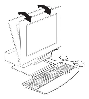
Dust buildup compounds problems associated with glare. Remember to clean your monitor screen periodically using a soft cloth moistened with a nonabrasive liquid glass cleaner.
