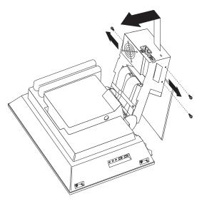
To remove the power supply, do the following:
