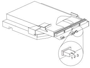
The slim CD-ROM drive and DVD drive are connected to the DASD interface board. The DASD interface board includes connectors for the two signal cables, power and speaker cables and jumper pins:
