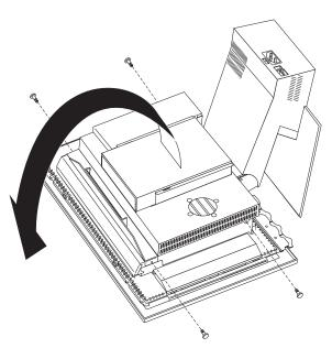
The rear EMC cover must be removed in order to remove the system board.
