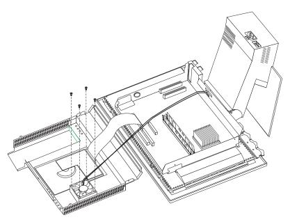
To remove the rear bucket housing-fan do the following:
