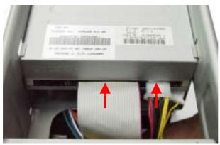
10. Connect the other end of the cable to the CD-ROM drive. Note the orientation of the cable before trying to connect it.
