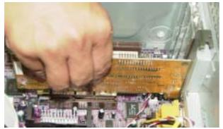
2. Following the figure, push the edge connector of the AGP card into the expansion slot.
