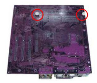
1. The plastic spacers provide extreme support in areas of high mechanical stress on your system board. Insert the plastic spacers in the 2 mounting holes as shown in the figure through the back of your system board. The plastic spacers are provided with the case.
