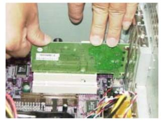
**6**.Gently use both hands to press down the Modem card onto the PCI slot.
