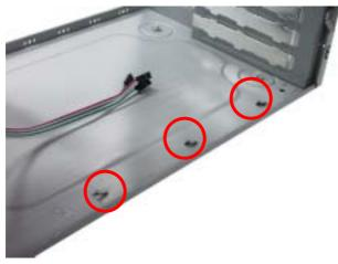
11. To install the system board inside the case. Locate the three mounting brackets on the case as shown in the figure.
