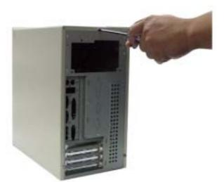
2.Locate the 3 screws at the back of the case; use the screwdriver to loosen them.
