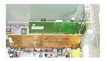
You have finished installing the Modem and AGP cards. Make sure that the add-on cards are installed properly on the system board See figure for reference.
