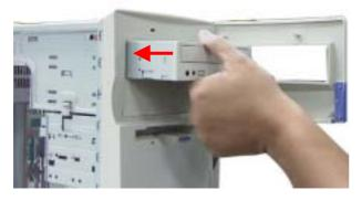
**5**. Slide the CD-ROM drive into the bay and align the drive's faceplate with the front of the case.
