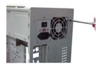
2. Using the screwdriver, gently tighten the three screws.
