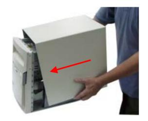
1. When all necessary peripherals and drivers are installed in the case and that there are no loose wires that may get in the way of the CPU fan and other components. Place back the top cover to the case.
