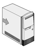
3 Align the screw holes and secure the cover with four screws.
