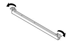
4 Insert the memory module by lining up the notches in the base of the module with the notches in the memory module on the system board. Slide the module between the guides on the side of the socket.
