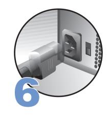
Verify voltage switch is set for your location. Plug in power cord to the computer and then to electrical outlet.
