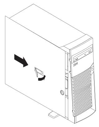
**Note:** If you removed the support bracket assembly after you removed the cover, reinstall it before you install the cover. For support bracket installation instructions, see "Removing the support bracket assembly" on page 46.
