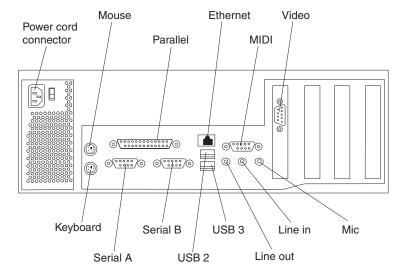
**Note:** If your computer is a SCSI model, the SCSI adapter will be located in PCI slot 1; the external connector will be located in the slot below the video connector on the tower model and to the right of the video connector on the desktop model. See "System and PCI extender board option connectors" on page 35 for the location of the PCI expansion slots.
