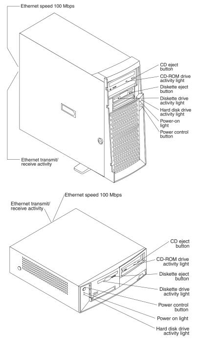
**CD eject button:** Push this button to open the CD tray to remove a CD from the drive.
