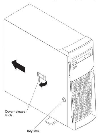
Complete the following steps to remove the side cover of the computer.
