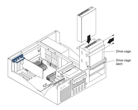
**Note:** If your computer has a CD-ROM drive installed in bay 1, remove the signal and power cables from the CD-ROM drive before rotating the drive cage out of the computer.
