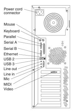
The following illustration shows the I/O connectors on the rear of the desktop model.
