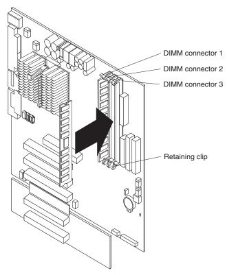
Complete the following steps to install a DIMM.
