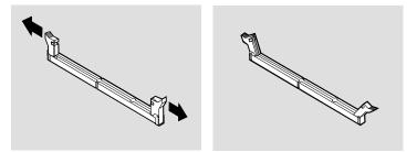
6. Position the new DIMM over the socket, making sure that the notches in the DIMM are aligned with the tabs on the socket. Push the DIMM straight down into the connector until the retaining clips close.
