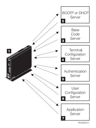
Figure 1. Network Station Power-On Sequence
