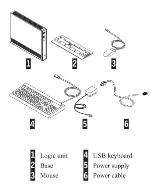
**2.** Attach the base to the logic unit.
