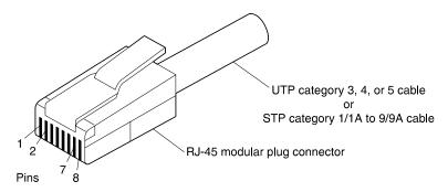
Figure 40. RJ-45 Connector
