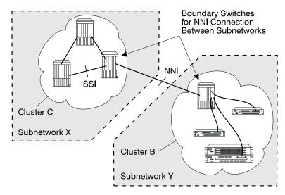
Figure 19. NNI Trunks Between Subnetworks
