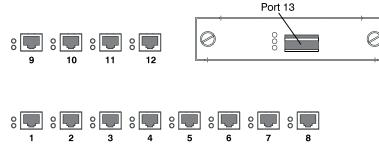
Figure 3. ATM Ports on the ATM Workgroup Switch Base Unit
