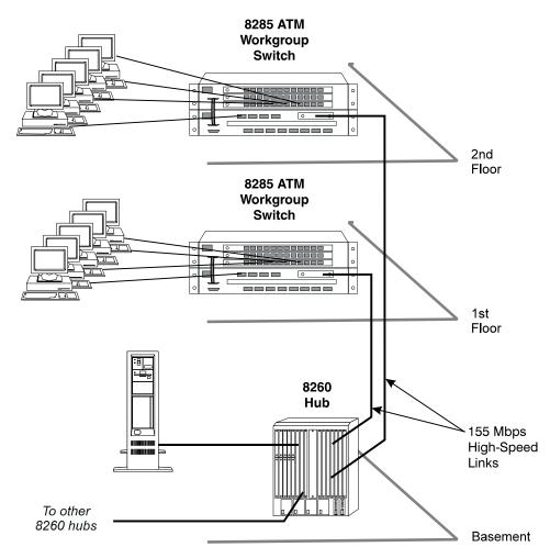
Figure 11. ATM Workgroup Switch in Floor Workgroup Configuration
