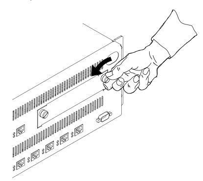
Figure 26. Removing the Dummy Slot Cover
