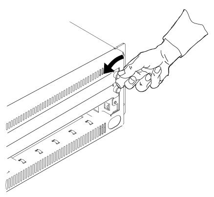
Figure 33. Removing the Dummy Module
