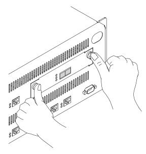
Figure 28. Pressing the I/O card into Place
