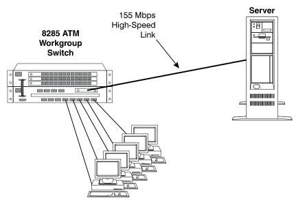
Figure 10. ATM Workgroup Switch in Client/Server Configuration
