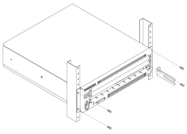
Figure 30. Rack Mounting the Expansion Unit
