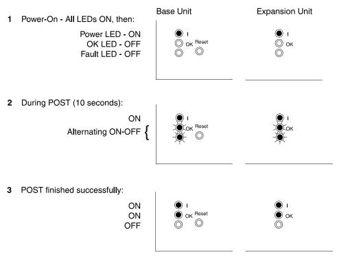
Figure 36. Pattern of the Status LEDs during Power-On Self-Test
