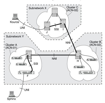
Figure 20. Example of Logical Links and Static Routes
