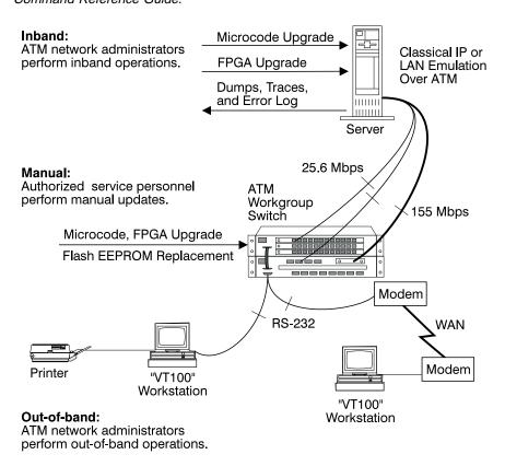
Figure 38. Upload and Download Operations for the ATM Workgroup Switch
