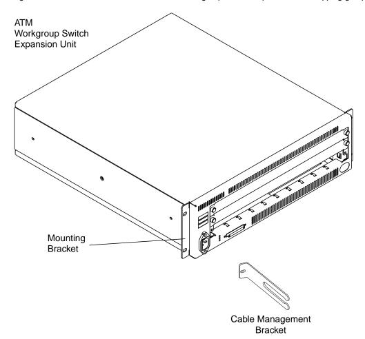
Figure 29. Contents of the Expansion Unit Shipping Group
