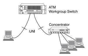
Figure 14. Connections to User Devices (UNI)
