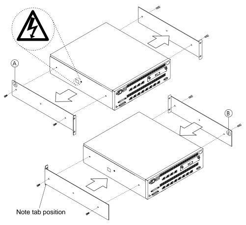
Figure 25. Attaching the Mounting Brackets for Surface Mounting
