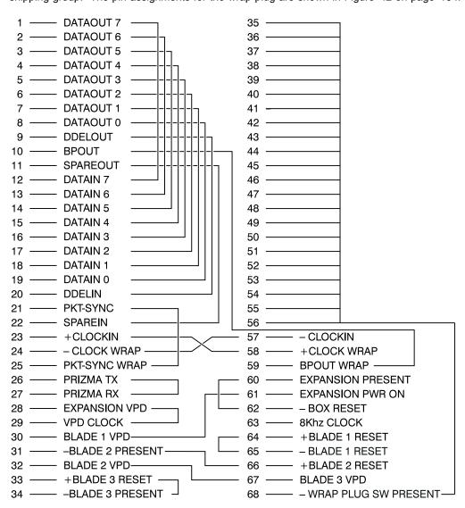
Figure 42. Pin Assignment: Expansion Connector Wrap Plug
