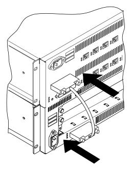
Figure 31. Attaching the Expansion Interface Cable
