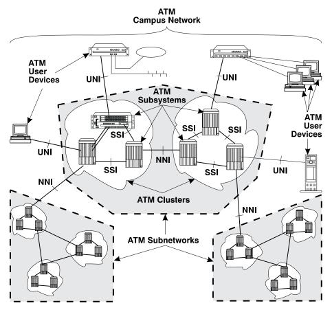
Figure 12. Components of an ATM Campus Network
