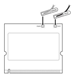
Plug the gray antenna cable with the tab marked "MAIN" into jack MAIN, and the black antenna cable with the tab marked "AUX" into jack AUX.
