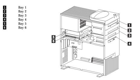
The drives in bays 5 and 6 must have nonremovable media. (In some models, the server comes with a hard disk drive in bay 6.) To install or remove drives in these bays, you must remove the rear (lower) drive cage.
