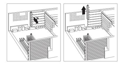
6. Touch the static-protective package that contains the adapter to any *unpainted* metal surface on the server; then, remove the adapter from the package.
