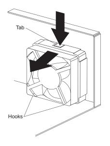
4. Press the tab and pull the front fan forward until it clears the server wall.
