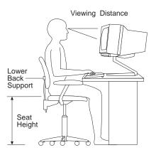
Adjust the monitor so the top of the screen is at, or slightly below, eye level. Place the monitor at a comfortable viewing distance,
