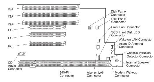
The following illustration shows the expansion slot connectors and other connectors on the riser card.
