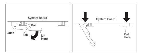
6. Using the tab, slide the system board out and set it aside.
