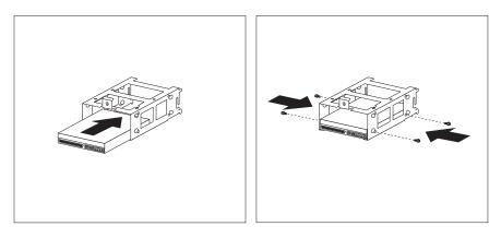
If your server does not come with a preinstalled hard disk drive, when you install the four screws that come with the drive, attach them to the drive from the bottom.
