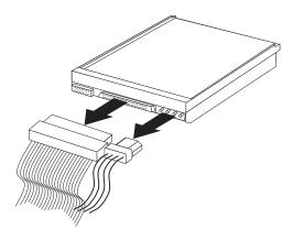
3. If you are removing a drive, remove the screws that hold the drive in the cage and slide the drive out of the cage.
