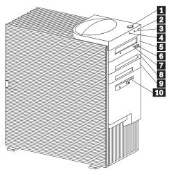
Your server comes with a diskette drive installed in bay 4 and a CD-ROM drive installed in bay 1. If your server comes with a hard disk drive, it is installed in bay 6.
