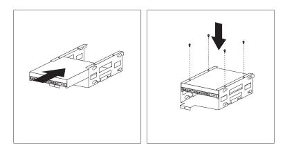
b. If you are installing a drive in bay 6, hold the drive with the connector side up before you slide it into the bay.
