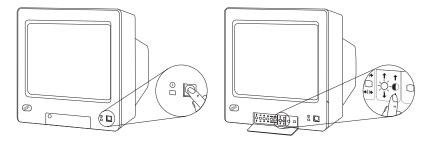
*Note:* The locations of the power switch and the Brightness and Contrast controls on your monitor might be different from those shown here.
