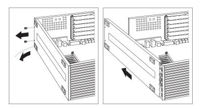
5. Slide the tabs on the end of the cover out of their openings and remove the cover.
