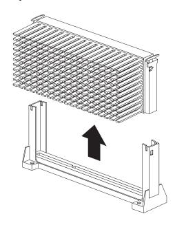
c. Lift the microprocessor out of the connector.
