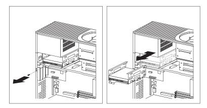
2. If there is a hard disk drive in bay 6, disconnect the cable from the drive in that bay. If there is a drive in bay 5, disconnect its cable.
