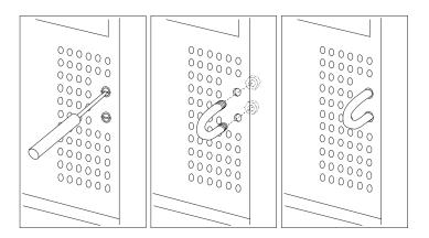
4. If you have completed installing the U-bolt and do not want to install any other internal options, replace the server side cover and reconnect all external cables and power cords. (See "Completing the Installation" on page 157 if you need additional information.) 5. Thread the cable through the U-bolt and around an object that is not a part of or permanently secured to the building structure or foundation, and from which it cannot be removed; then, fasten the cable ends together with a lock.
