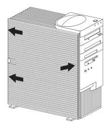
5. If a cover lock is present, go to the back of the server and lock the cover.
