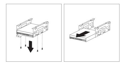
4. If you are installing a drive, slide the drive into the bay and secure it with the screws.
