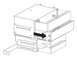
3. Touch the static-protective package containing the new drive to any *unpainted* metal surface; then, remove the drive from it.
