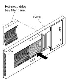
Figure 12. Removing the hot-swap drive bay filler panel from the bezel
