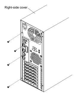
Figure 10. Removing the right-side cover
