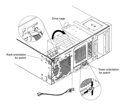
Figure 6. Relocating the power-switch and LED panel
