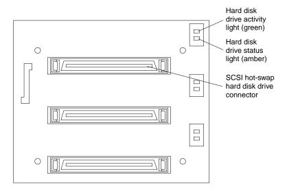
**Note:** The hard disk drive activity light and hard disk drive status light on the backplane match the hard disk drive activity light and hard disk drive status light on the hot-swap drive.
