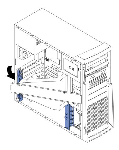
Do the following to remove the support bracket assembly:
