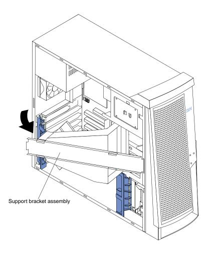
Figure 2. Removing the support bracket assembly
