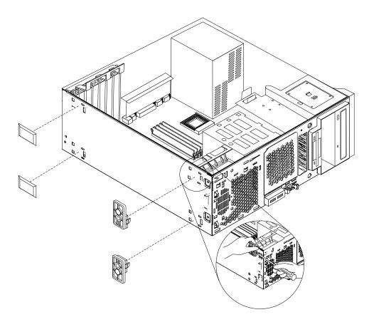
Figure 5. Removing the system feet
