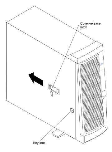
Figure 1. Removing the left-side cover
