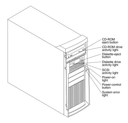
**CD-ROM eject button:** Press this button to release a CD from the drive.
