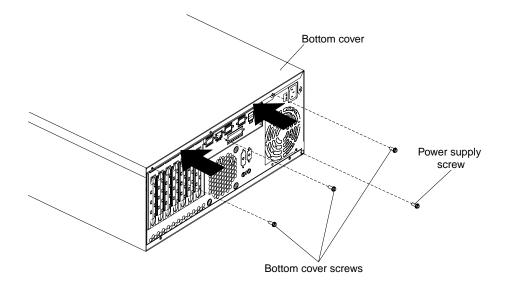
Figure 11. Installing the new bottom cover
