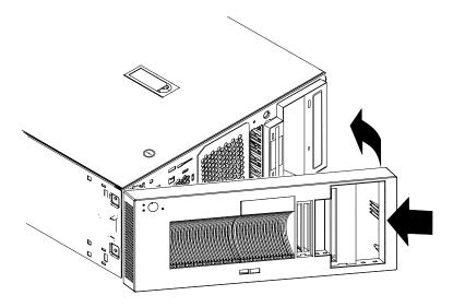
Figure 14. Installing the new system bezel
