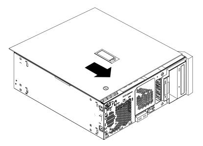
Figure 7. Installing the top cover
