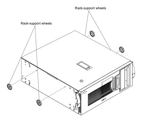
Figure 16. Attaching the rack-support wheels
