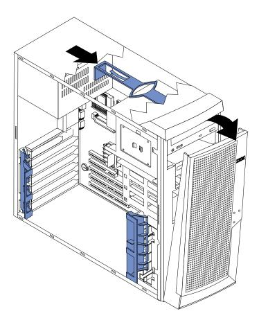
Figure 3. Removing the front door and bezel assembly
