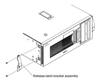
Figure 15. Installing the release-latch-bracket assemblies
