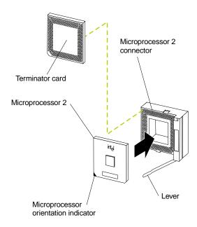
**Attention:** To avoid bending the pins, do not use excessive force when pressing the microprocessor into the connector.
