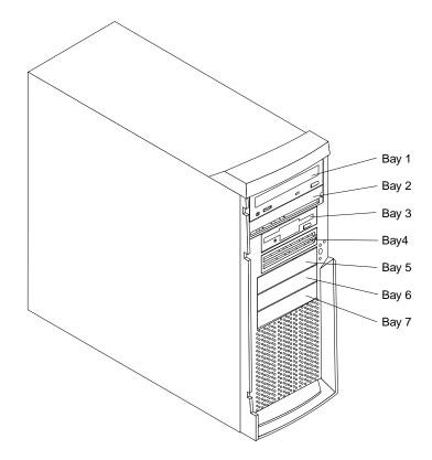
To remove or install a drive, you must turn off the server first, unless you are removing or installing a hot-swap hard disk drive. Diskette drives, tape drives, and CD-ROM drives are removable-media drives. You can install removable-media drives in bays 1, 2, 3, and 4. You can install SCSI hard disk drives in bays 4, 5, 6, and 7.
