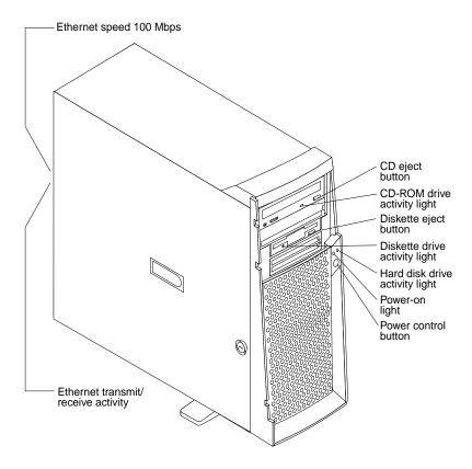
**CD** eject button: Push this button to open the tray to insert or remove a CD.
