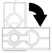
When you are finished installing options and have reinstalled the side cover, turn the two front stabilizing feet a quarter turn out from the server and set it carefully back on its feet.
