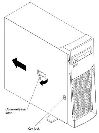
Complete the following steps to remove the side cover of the server.
