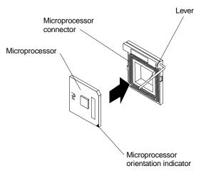
**Note:** Do not use excessive force when pressing the microprocessor into the connector.
