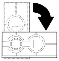
When you need to access the inside of the server to install options, you might find it easier to place the server on its side, so that the system board is facing you. If you do so, rotate the feet in towards the server, so that they do not break off due to the weight of the server.
