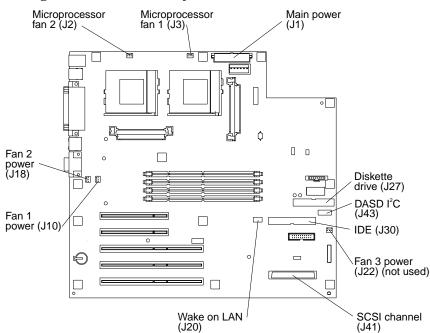
The following illustration identifies system-board connectors for internal cables.
