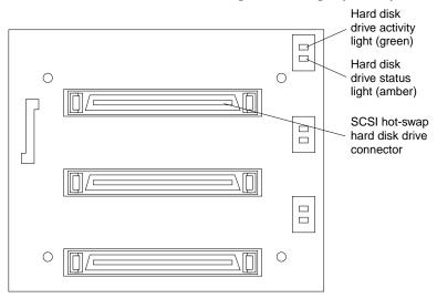
The hard disk drive activity light and hard disk drive status light on the backplane match the hard disk drive activity light and hard disk drive status light on the hot-swap drive.
