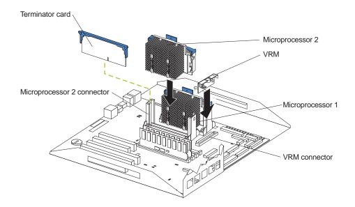
To install an additional microprocessor:
