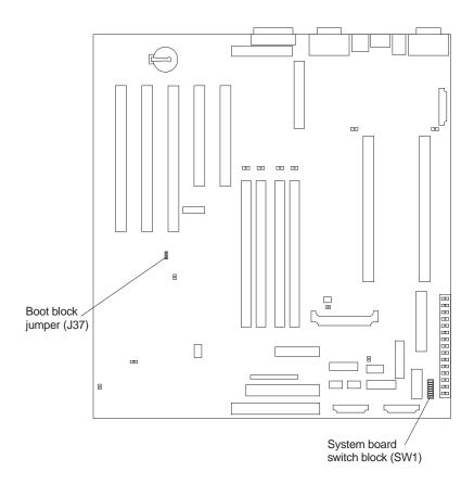
**Note:** Any jumper blocks on the system board that are not shown in the illustration are reserved. For normal operation of the system, no jumpers should be installed on any of the jumper blocks.
