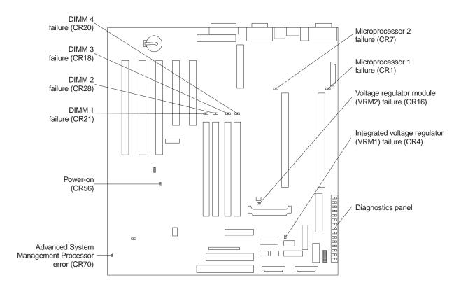
**Note:** The power-on LED is lit when system power is present in the server.
