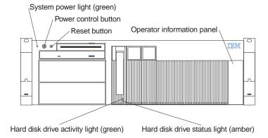
**System power light:** When this green light is on, system power is present in the server. When this light flashes, the server is in standby mode (the system power supply is turned off and AC current is present). When this light is off, either a power supply, AC power, or a light has failed.
