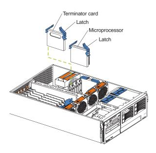
To install an additional microprocessor:
