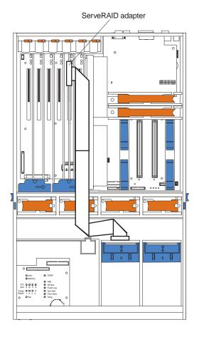
11. Install the ServeRAID adapter in the desired PCI slot. See "Installing a hot-plug adapter" on page 69 for adapter installation instructions. Refer to the ServeRAID adapter option documentation for additional information on installing a ServeRAID adapter in the
