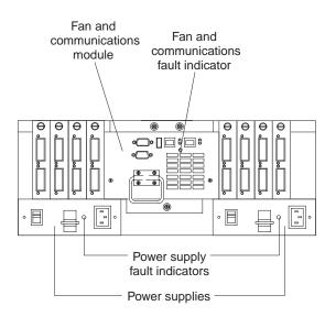
The storage-management software causes the fault indicator to light before the temperature has risen sufficiently to shut down the power supplies. The light comes on when the controller unit temperature exceeds 45&dreg. C (113&dreg. F). The controller unit shuts down if the temperature rises to 70&dreg. C (158&dreg. F). If both power supplies shut down, the fault indicator cannot come on.
