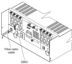
3. Insert the protective cap on the GBIC.
