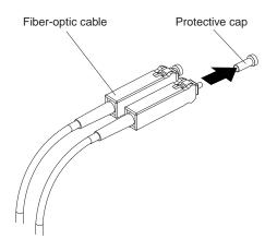
2. Connect the fiber-optic cable to a GBIC that is installed in a mini-hub.
