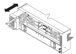
b. Unlock and open the controller levers; then, using the levers, pull the controller out a couple of inches. Grasp both sides of the controller and remove it.
