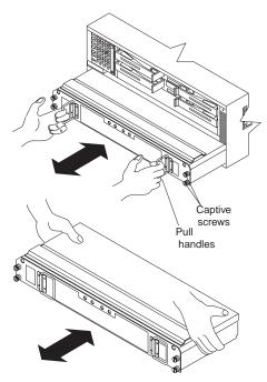
Using the pull tab handle, lift up and pull to release each power supply; then, slide out the power supply.
