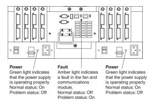
The mini-hub indicator lights on the back of the controller unit are shown in the following illustration.
