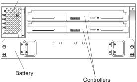
The following illustration shows the controller unit back view.
