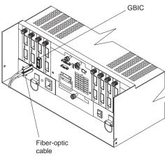
2. Remove any GBICs in the mini-hub. If a GBIC you are removing has a metal latch, move the latch to the unlocked (center) position. Pull the GBIC from its mini-hub port; then, replace the protective caps on the GBIC.
