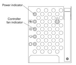
When the controller fan is operating properly, the green power indicator is on and the amber indicator is off.
