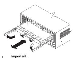
To prevent data loss, replace controller A in the upper solt and controller B in the lower slot.
