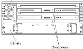
**Back view:** The following two illustrations show the controller unit back view and the following components:
