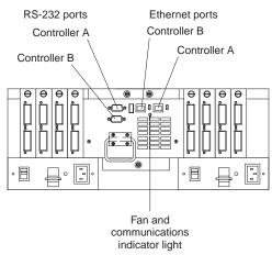
4. Remove the failed fan and communications CRU from the controller unit.
