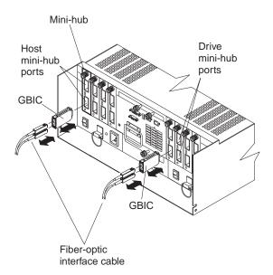
**Controller unit interface ports:** The host and drive GBIC mini-hub ports are used to attach cables from the controller and drive enclosures to the storage subsystem. There are also Ethernet ports for storage subsystem- management and RS-232 (serial) ports for diagnostic services. The controller unit interface ports are shown in the following illustration.
