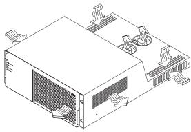
The controller unit must have proper air circulation throughout the chassis. To boost air circulation, the chassis has air vents along its top and sides. These vents serve as air intake and exhaust passages. Assure that vents are clean and free of obstruction.
