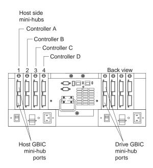
**Drive mini-hubs:** Each drive mini-hub connects to Controller A and Controller B and each drive mini-hub represents a single drive channel. The drive channels are set up in pairs to support redundant drive loop configurations (two data paths per drive enclosure). Each pair supports up to 11 drive enclosures, containing 10 drives each, or a maximum of 110 drives. A fully configured controller unit supports a maximum of 22 drive enclosures (11 drive enclosures per channel pair), or 220 drives.
