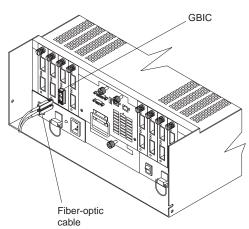
2. Remove the GBICs from the mini-hub ports. If the GBIC you are removing has a metal latch, move the latch to the unlocked (center) position. Pull the failed GBIC from its mini-hub port.
