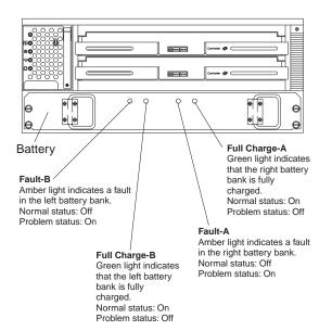
The indicator lights on the back of the controller unit are shown in the following two illustrations.
