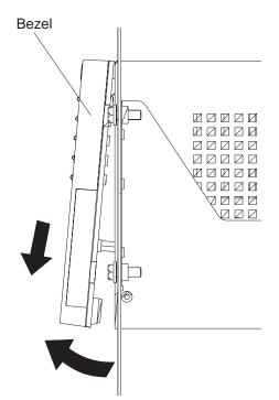
2. To replace the bezel, slip the top edge of the bezel under the lip on the chassis, then push the bottom of the bezel until the pins snap into the mounting holes, as shown in the following illustration.
