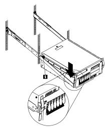
Slide the server backward or forward as necessary until the notches meet.
