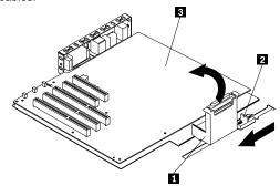
While tilting the cable bracket 1 forward, slide the system board/backplate assembly latch 2 in the direction shown. Then, remove the system board/backplate assembly 3 out of the server.
