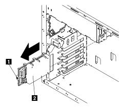
5. Release the power backplane/backplate assembly latch 1; then, slide the power backplane/backplate assembly 2 out of the server.
