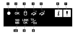
System Power Light: When this green light is on, system power is present in the server. When this light flashes, the server is in standby mode (the system power supply is turned off and AC current is present). When this light is off, either a power supply, AC power, or a light has failed.
