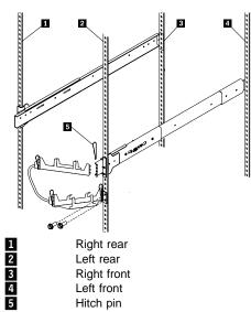
Attach the free end of the cable-management arm to the rear of the left slide rail, using a hitch pin 5.
