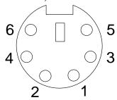
The following table shows the pin-number assignments for the connector used by the auxiliary-device port.
