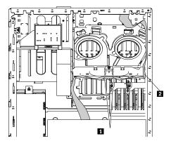
f. Reattach the cable to the operator LED panel.
