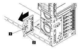
Release the SCSI backplane assembly latch then, slide the SCSI backplane assembly out of the server.
