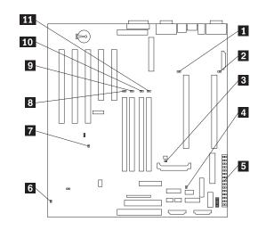
**1** Secondary microprocessor failure (CR7)
