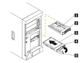
**1** Filler panel for use with half-high drives (tray and slim filler bezel)
