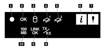
**System Power Light:** When this green light is on, system power is present in the server. When this light flashes, the server is in standby mode (the system power supply is turned off and ac current is present). When this light is off, either a power supply, ac power, or a light has failed.
