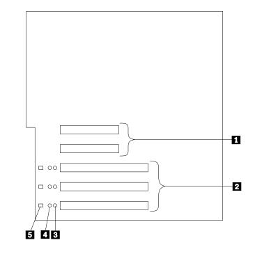
The following illustration shows the location of the PCI expansion slots on the system board.
