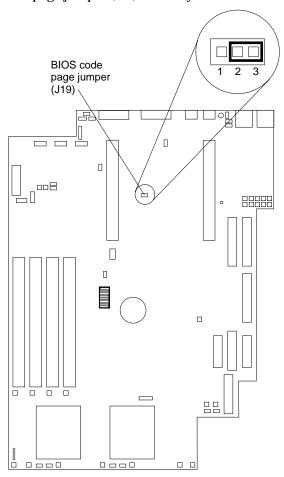
3. Place a jumper on pins 1 and 2 to enable the BIOS back page.
