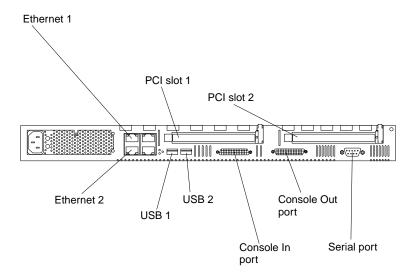
This section provides information about the input/output (I/O) ports on your server. These ports include the following:
