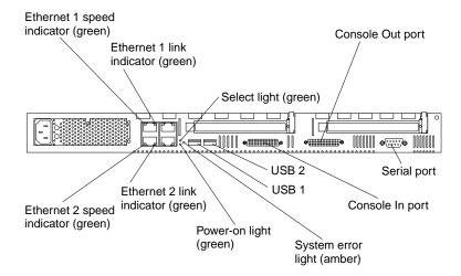
**Ethernet 1 speed indicator:** This green LED lkights when the speed of the Ethernet LAN that is connected to the Ethernet port 1 is 100Mbps.
