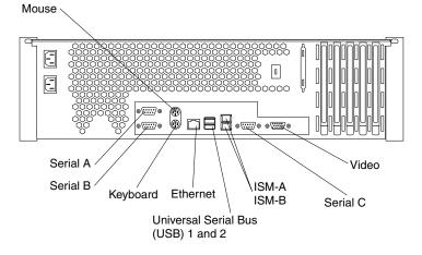
Future releases of the Integrated System Management (ISM) firmware code will enable the Integrated System Management processor to send or forward alerts to IBM system management adapters using the ISM ports. Future releases of the Integrated System Management (ISM) firmware code will enable the Integrated System Management processor to send or communicate using a modem and this dedicated serial port.
