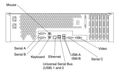
Future releases of the Integrated System Management (ISM) firmware code will enable the Integrated System Management processor to communicate using a modem and the dedicated Serial C port.
