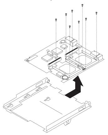
Reverse these steps to install the replacement I/O board.
