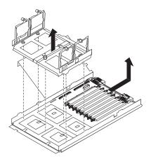
Note the alignment of the heat-sink retention bracket (the arrow on the bracket aligns with the arrow on the processor board). You will need to align the bracket the same way when reinstalling it.
