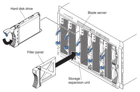
Attention: To maintain proper system cooling, do not operate the BladeCenter unit for more than 1 minute without either a hot-swap hard disk drive or a filler panel installed in each storage expansion unit bay.
