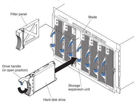
Complete the following steps to install a drive in a storage expansion unit.
