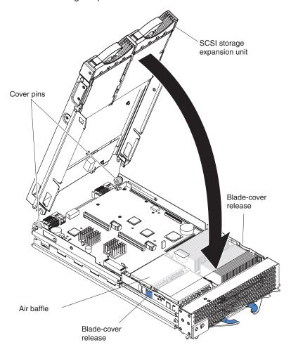
b. Lower the storage expansion unit so that the slots at the rear slide down onto the pins at the rear of the blade server.
