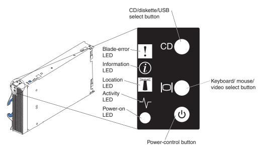
**CD/diskette/USB select button:** Press this button to associate the CD-ROM drive, diskette drive, and USB port with this blade server. The LED on this button flashes while the request is being processed, then is steady when the ownership of the CD-ROM drive, diskette drive, and USB port has been transferred to this blade server. It can take approximately 20 seconds for the operating system in this blade server to recognize the CD-ROM drive, diskette drive, and USB port.
