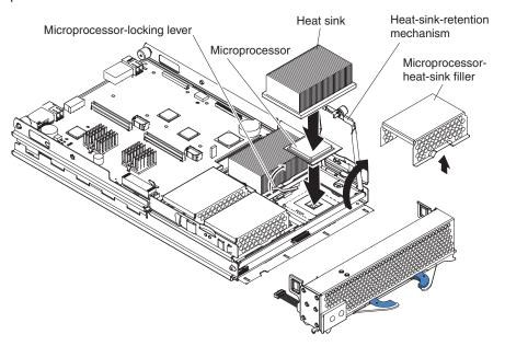
Complete the following steps to install an additional microprocessor:
