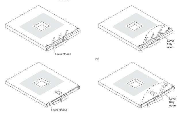
d. Center the microprocessor over the microprocessor socket. Align the triangle on the corner of the microprocessor with the triangle on the corner of the socket, and carefully press the microprocessor into the socket.
