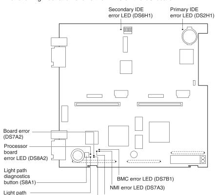
The following illustration shows the LEDs on the I/O board.
