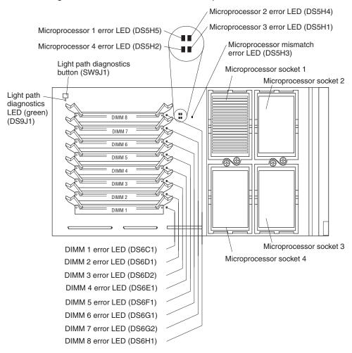
The following illustration shows the LEDs on the I/O board.
