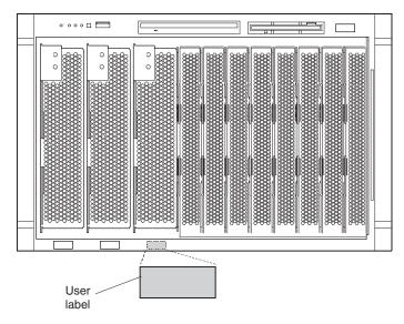
**Important:** Do not place the label on the blade server or block the ventilation holes on the blade server in any way.
