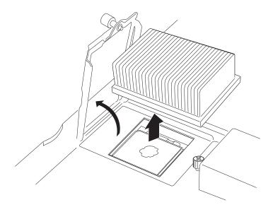
8. Rotate the locking lever on the microprocessor socket from its closed and locked position until it stops or clicks in the fully open position (approximately 135° angle), as shown.
