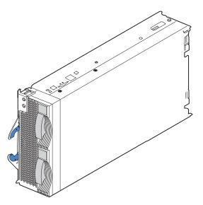
9. Insert the combined blade and expansion unit into three adjacent BladeCenter unit bays.
