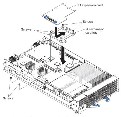
Complete the following steps to install an I/O expansion card:
