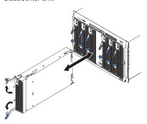
The following illustration shows how to remove the blade server from the BladeCenter T unit.
