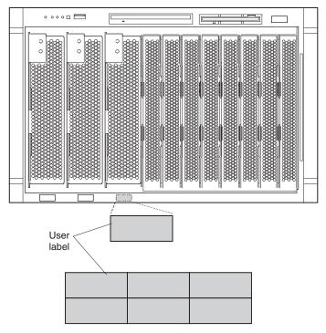
**Important:** Do not place the label on the blade server itself or in any way block the ventilation holes on the blade server.
