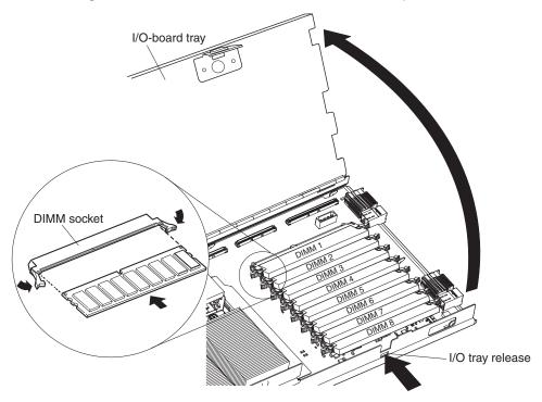
Complete the following steps to install a DIMM:
