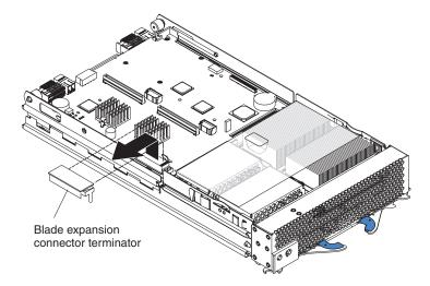
6. Before installing the SCSI storage expansion unit, check that all components are installed and seated correctly and that you have not left loose tools or parts inside the blade server.
