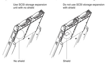
a. Orient the storage expansion unit as shown in the illustration.
