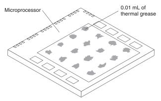
Note: 0.01 mL is one tick mark on the syringe. If the grease is properly applied, approximately half (0.22 mL) of the grease will remain in the syringe.
