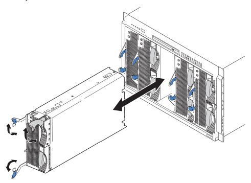
**Note:** When any blade server or option is in blade bay 7 through 14 (in the BladeCenter unit) or blade bay 5 through 8 (in the BladeCenter T unit), power modules must be present in all four power bays.
