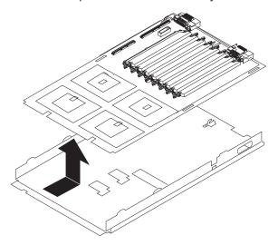
Reverse these steps to install the replacement processor board.
