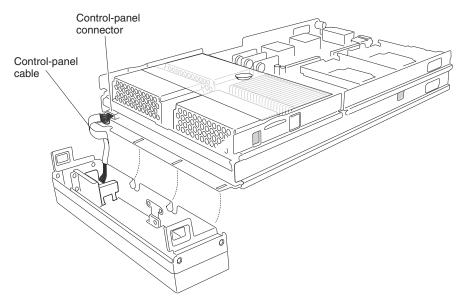
3. Insert the tabs on the bottom of the bezel up into the matching holes on the server chassis; then, rotate the top of the bezel toward the server until the tabs at the top of the bezel snap into place.
