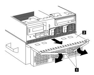
4. Open the two latches **1** at the top of the processor housing assembly **2** . Fully extend the latches.
