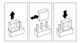
4. Slide the jumper fully onto these pins.
