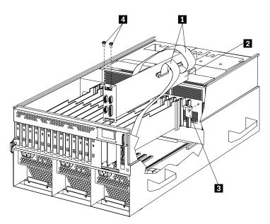
b. Disconnect all cables 1 from the I/O function card 2. Note carefully where each cable is connected before you remove it. See "I/O function
