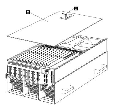
4. Close the cover-release latch to pull the cover forward and lock the cover in place.
