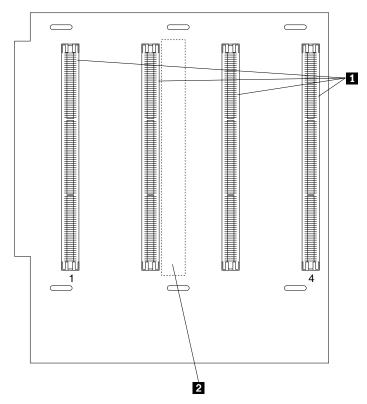
Processor or processor terminator card connectors (A1–A4 or B1–B4)
