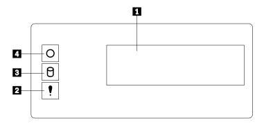
Information message panel: System monitor information appears on this display. The Advanced System Management PCI adapter monitors system functions and generates the messages. See "System-monitoring messages" on page 146 for more information.
