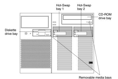
Your server contains hardware and an operating system that support the replacement of a failed hard disk drive without turning off the server, when the drive is connected to a ServeRAID adapter. Therefore, you can continue to operate your system while a hard disk drive is removed or installed. These drives are known as hot-swappable drives. They are also referred to as hot-swap drives.
