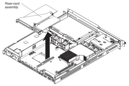
**Attention:** PCI expansion-slot covers must be installed on all vacant slots. This maintains the electronic emissions characteristics of the server and ensures proper cooling of server components.
