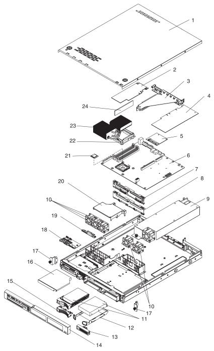
**Attention:** Do not remove the preinstalled air deflector unless directed to do so in this publication or by IBM Service. See the illustration on page 87 for the location of the air deflector in the server. An air deflector comes in Misc. kit 2 in the following list.
