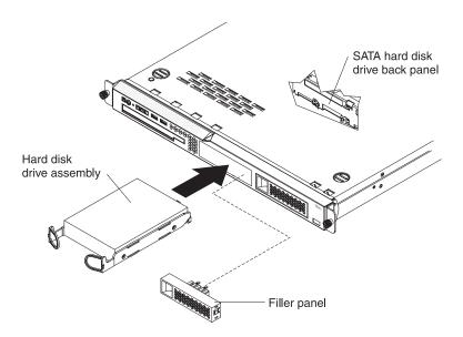
**Attention:** To avoid damage to the hard disk drive connectors, make sure that the server cover is in place and fully closed whenever you install or remove a hard disk drive.
