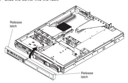
5. To install the bezel, if it was removed, tilt the bezel and align the latches with the slots at each front corner of the chassis; then, straighten the bezel and snap it into place.
