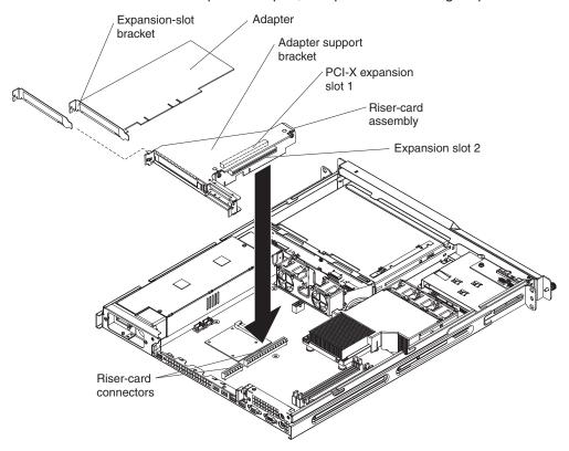
**Note:** Depending on the riser card that is installed, expansion slot 2 is either a PCI-X or a PCI-Express slot.
