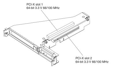
The following illustration shows the location of the PCI-X and PCI Express slots on the riser-card assembly option.
