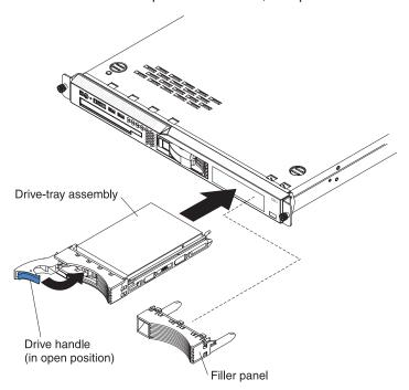
**Attention:** To avoid damage to the hard disk drive connectors, make sure that the server cover is in place and fully closed whenever you install or remove a hard disk drive.
