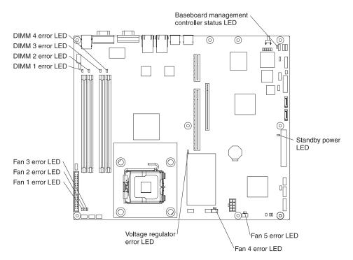
The baseboard management controller status LED flashes to indicate that the mini-BMC is functioning normally.
