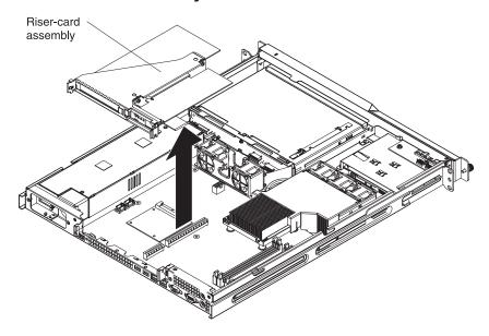
Complete the following steps to remove the riser-card assembly:
