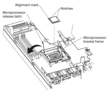
**Attention:** The microprocessor contacts are fragile; handle the microprocessor very carefully.
