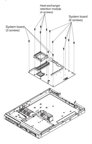
To remove the system board, complete the following steps:
