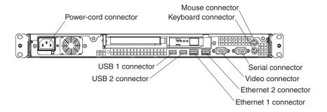
**Power-cord connector:** Connect the power cord to this connector.
