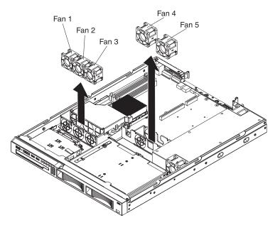
8. Position the replacement fan so that the airflow arrow on the side of the fan is pointing toward the rear of the server.
