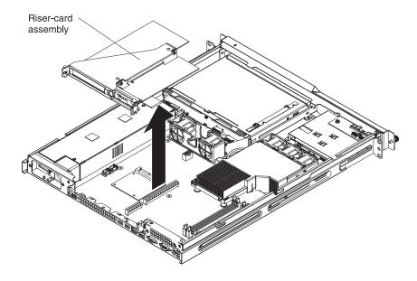
Complete the following steps to install the riser-card assembly.
