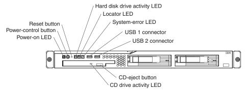
**Power-on LED:** When this LED is lit, it indicates that the server is turned on. When this LED is off, it indicates that ac power is not present, or the power supply or the LED itself has failed.
