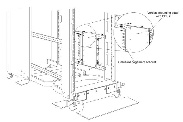
Figure 23. Installing a PDU vertically in a rack cabinet
