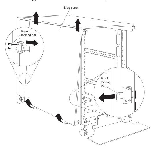
Figure 8. Removing the NetBAY25 side panels
