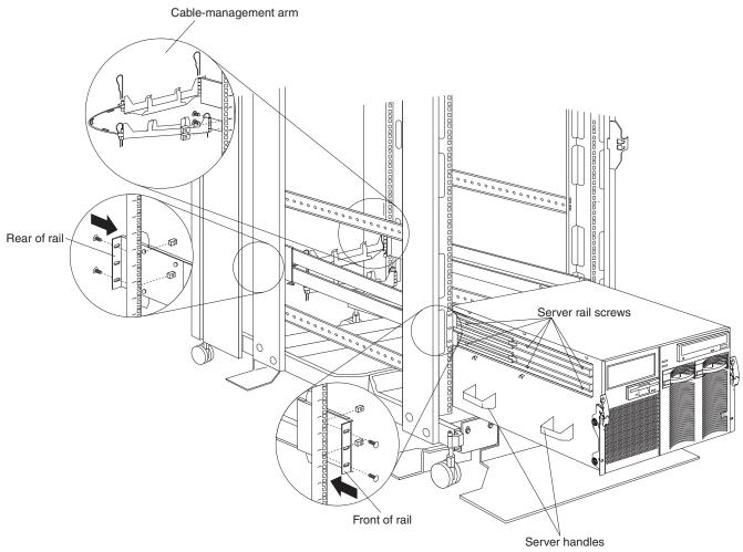
Figure 25. Installing a large server
