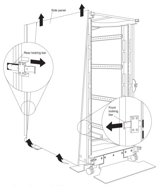
Figure 10. Removing the NetBAY42 side panels
