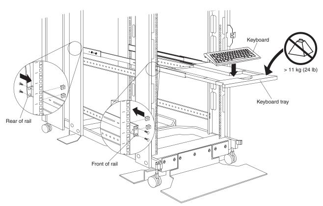
Figure 32. Installing a keyboard tray and keyboard
