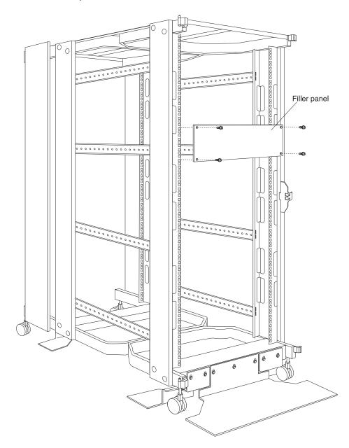
Figure 38. Installing a blank filler panel
