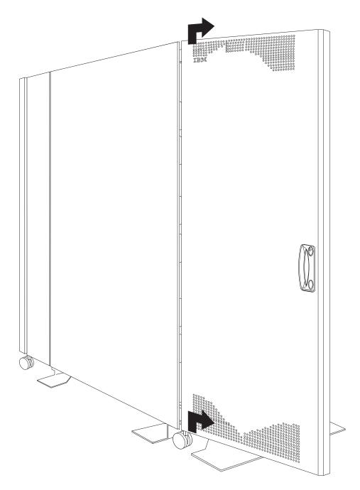
Figure 13. Removing a front door from the NetBAY42 rack cabinet
