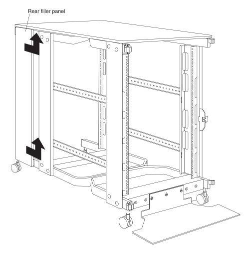
Figure 9. Removing the NetBAY25 rear filler panels
