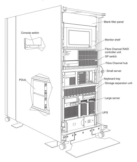
Figure 19. Installing optional devices in the NetBAY42 Rack cabinet
