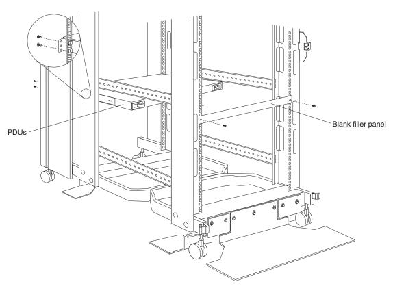
Figure 24. Installing a PDU horizontally in a rack cabinet
