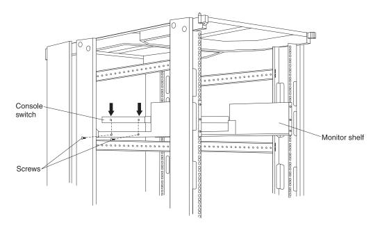
Figure 35. Installing a console switch in a monitor shelf
