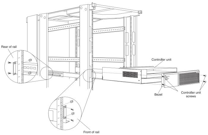
Figure 28. Installing a Fibre Channel RAID controller unit
