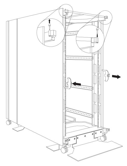
Figure 14. Moving the hinge pins and front door latch
