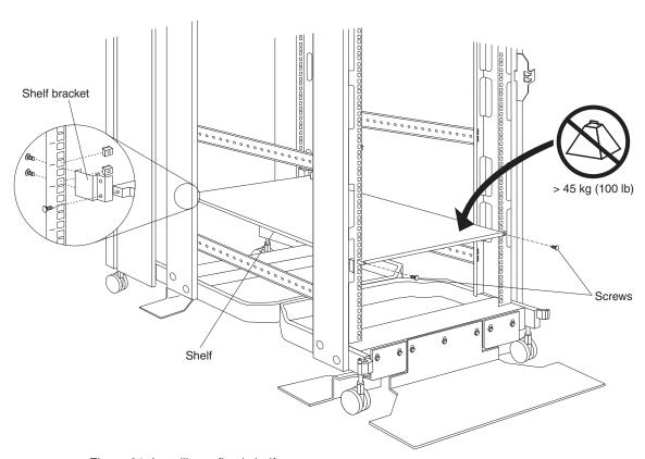
Figure 31. Installing a fixed shelf
