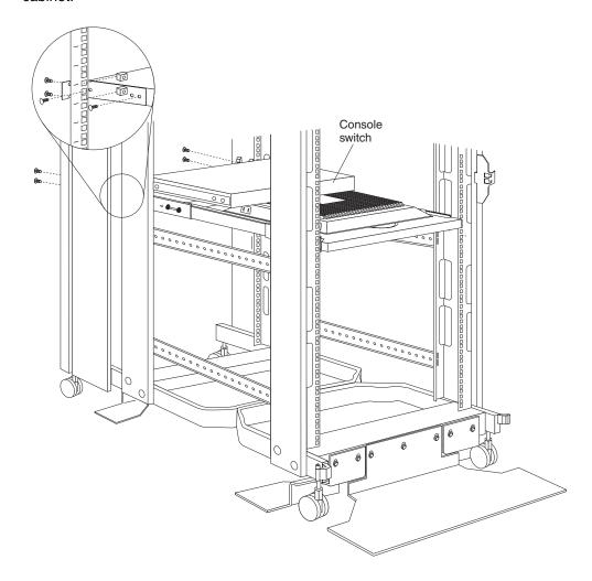
Figure 37. Installing a console switch horizontally
