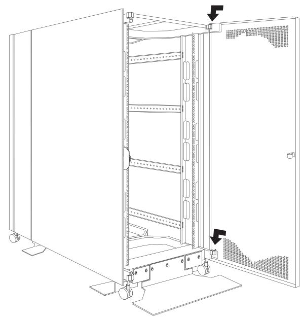
Figure 15. Rotating and installing the door
