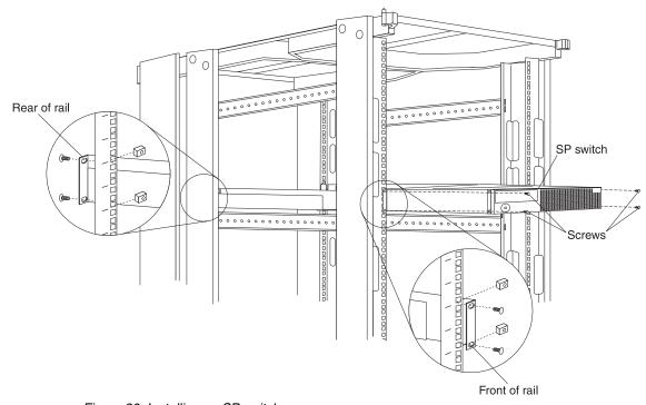
Figure 30. Installing an SP switch
