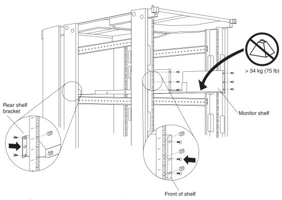
Figure 34. Installing a monitor shelf
