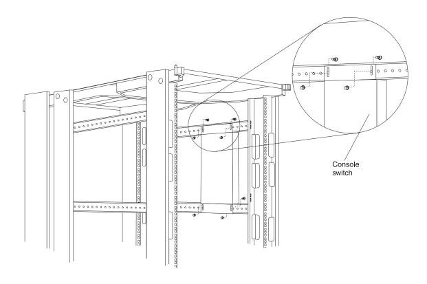
Figure 36. Installing a console switch vertically
