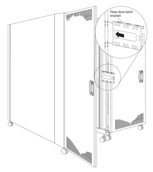
Figure 18. Installing the rear-door-latch-bracket on a rack cabinet
