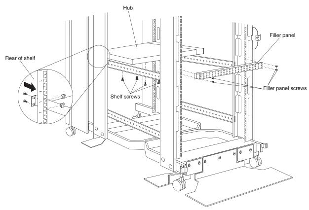
Figure 29. Installing a Fibre Channel hub
