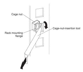
Figure 20. Installing cage nuts with the cage-nut-insertion tool
