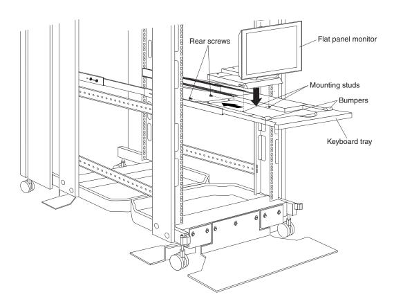
Figure 33. Installing a flat panel monitor rack mount kit
