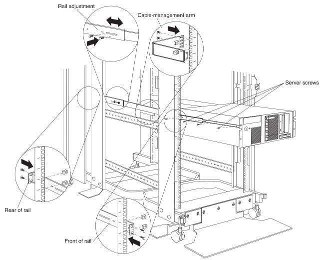
Figure 26. Installing a small server
