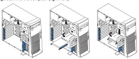
**Note:** Clear any cables that might impede the replacement of the drive cage.
