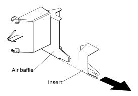
4. Remove the air-baffle insert from the air-baffle assembly before you install the additional microprocessor. Store the air-baffle insert in a safe place for future use.
