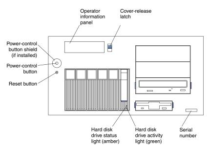
**Power-control button shield:** You can install this circular disk over the powercontrol button to prevent accidental manual power-off. This disk is provided with your server.
