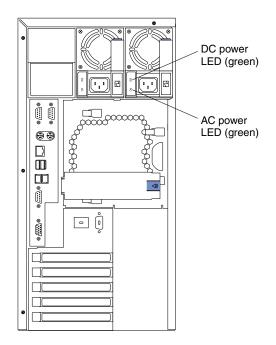
**AC power light:** This green light provides status information about the power supply. During typical operation, the ac power light is on. For any other combination of lights, see "Power-supply LEDs" on page 111.
