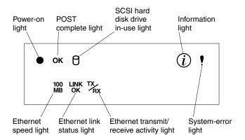
**Power-on light:** This green LED lights when system power is present in the server. When this light flashes, the server is in Standby mode (the system power supply is turned off and current is present). If this light is not on, the power cord is not connected, the power supply has failed, or this LED has failed. See Chapter 6, "Solving Problems," on page 85.
