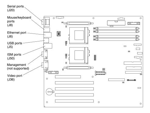
**Note:** ISM ports (ISM A and B) are used for the RS-485 interconnect network communications.
