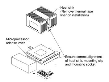
Make sure the heat-sink guide fits between the microprocessor and the microprocessor socket.
