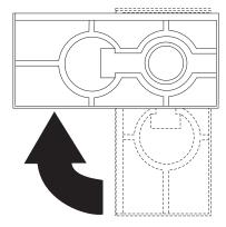
When you need to access the inside of the server to install options, you might find it easier to place the server on its side, so that the system board is facing you. If you do so, rotate the feet in towards the server, so that they do not break off due to the weight of the server.
