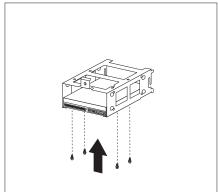
6. Reinstall the lower drive bracket and secure it with the screw.
