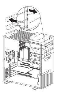
b. Remove the top cover by using a flat-blade screwdriver to release the tab on the left edge, as shown.
