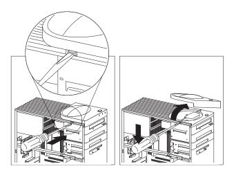
c. Disconnect the power and signal cables attached to the drives in the upper drive bracket.
