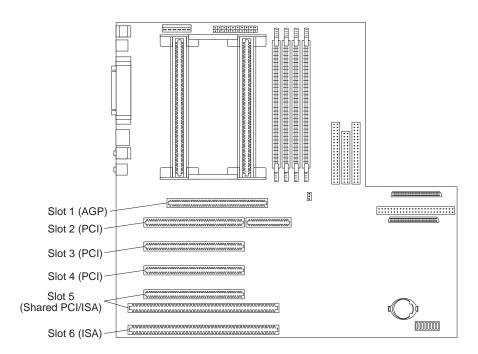
Note: Expansion slot 5 is a shared slot. Shared slots can be occupied by an adapter attached to either the PCI slot connector or the adjacent ISA slot connector, but not both.
