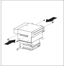
9. Reinstall the upper drive bracket and secure it with screws at the top and bottom.
