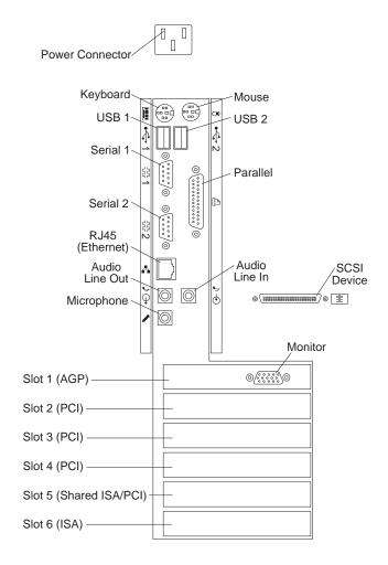
**Power Connector:** The server power cable connects here.
