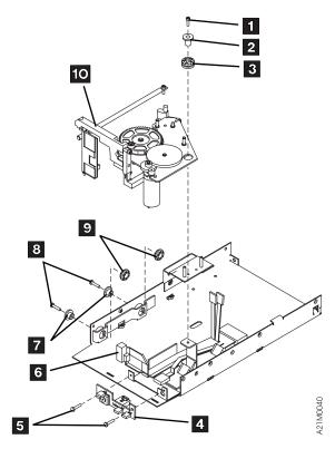
Figure 326. Drive Loader Assembly Exploded View
