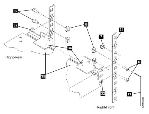
Figure 189. Support Slide, right side, Models C21 and C22
