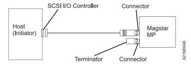
Figure 198. Example of Attaching One SCSI Device to the Host (Initiator)
