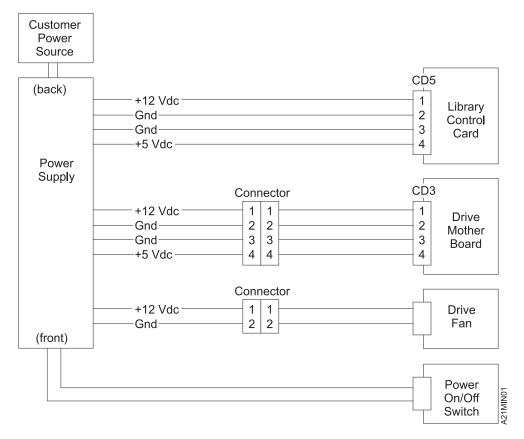
Figure 26. Power Block Diagram
