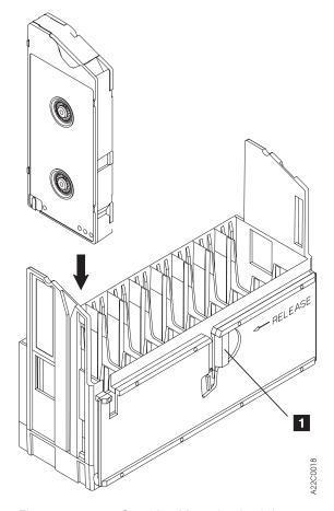
Figure 52. 3570 Cartridge Magazine Lock Lever
