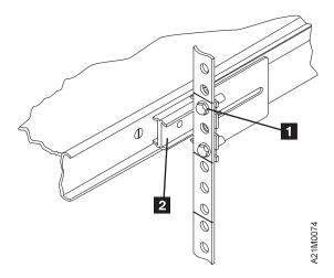
Figure 206. Inner Slide to Rack Clearance
