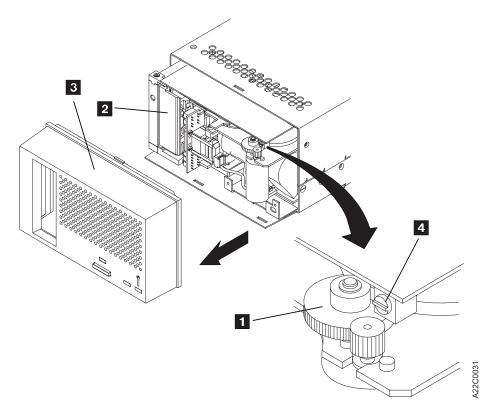
Figure 252. Removing a Stuck Cartridge From a Drive
