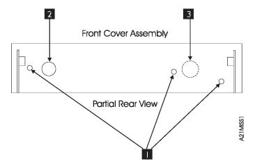
Figure 282. Library Front Door Assembly—Rear View Holding Screws
