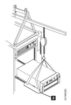
Figure 209. Raising 3570 Using Hoist
