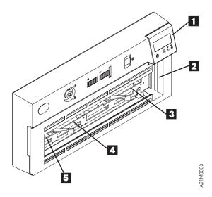
Figure 49. Magazine and Cartridge Locations, Models C01, C02, C11 and C12
