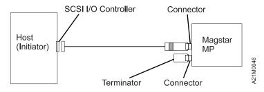
Figure 225. Example of Attaching One SCSI Device to the Host (Initiator)
