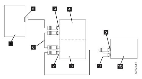
Figure 229. Example of Attaching Multiple SCSI Devices to a Host (Initiator)
