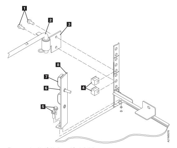
Figure 207. Attaching Cable Arm and Strain Relief
