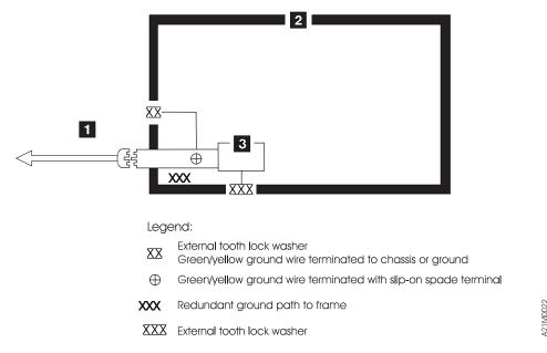
Figure 182. AC Grounding Diagram (50 Hz and 60 Hz)
