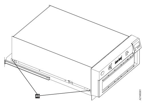
Figure 210. Attaching the 3570 to the Rack Tray
