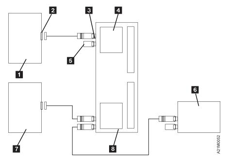
Figure 230. Attaching 3570 Models C02 or C12 In Split Configuration
