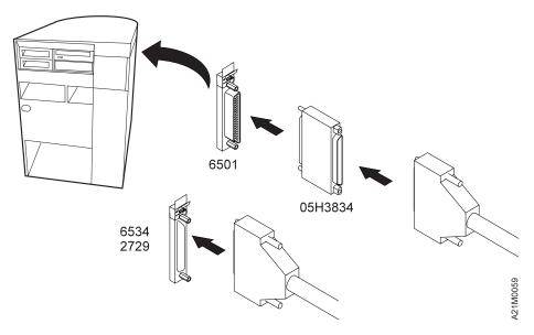
Figure 41. SCSI System Cable Attachment at the AS/400 Host (Initiator)
