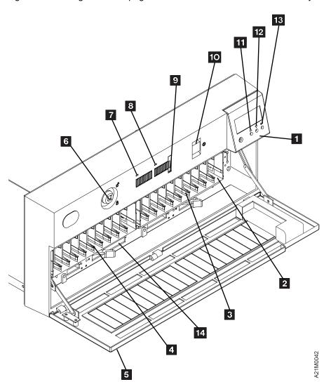
Figure 53. Front Assembly for Model C01, C02, C11, and C12
