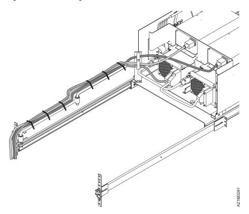
Figure 239. Cable length adjusting Models C11 and C12
