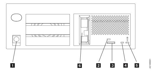
Figure 44. Model C00 Drive Operator Controls
