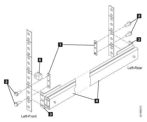
Figure 186. Support Slide, left side, Models C11 and C12
