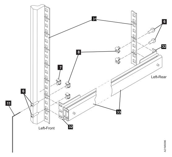
Figure 187. Support Slide, left side, Models C21 and C22
