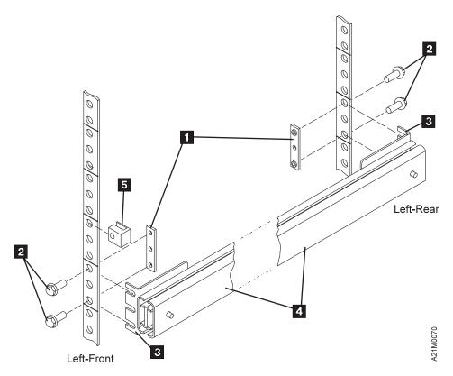
Figure 203. Attaching Left-hand Slide and Bracket assembly
