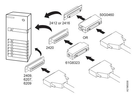
Figure 40. SCSI System Cable Attachment at the RS/6000 Host (Initiator)
