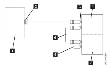
Figure 228. Example of Attaching One SCSI Device to the Host (Initiator)
