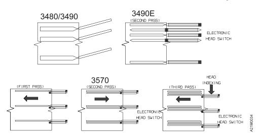
Figure 17. Serpentine Interleaved Track Sets
