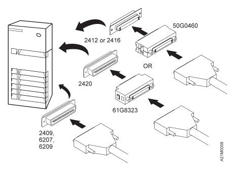
Figure 222. Installing the SCSI System Cable at the RS/6000 Host (Initiator)
