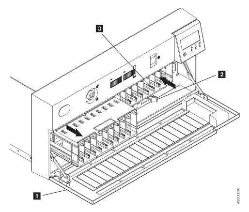
Figure 250. Loaded and unloaded Magazine (with the Door in the Open Position)
