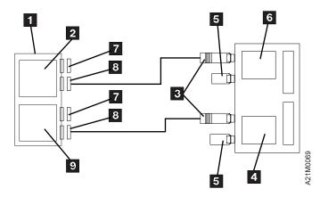
Figure 235. AS/400 FC 6501—Split Configuration (single host, two IOPs)
