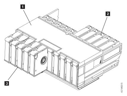
Figure 39. 3570 Cartridge Magazine
