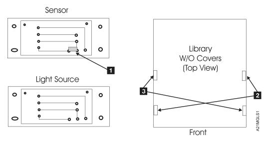
Figure 330. Library Global Sensor Component Identification and Locations
