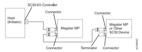
Figure 199. Example of Attaching Multiple SCSI Devices to the Host
