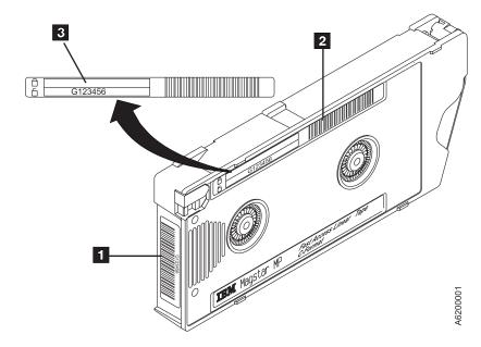
Figure 256. Magstar MP Tape Cartridge Labels
