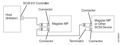
Figure 226. Example of Attaching Multiple SCSI Devices to the Host
