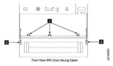
Figure 283. Library Front Door Assembly—Front View Holding Screws
