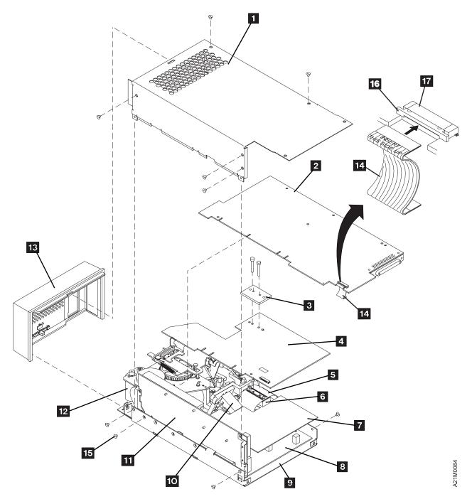
Figure 317. Base Drive FRU Breakout
