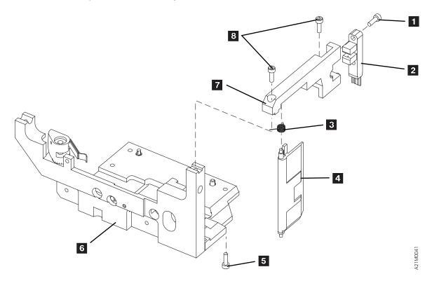
Figure 327. Drive Loader Front Components Exploded View
