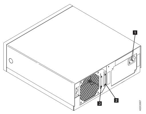
Figure 200. Drive-Only Model C00 SCSI Connection
