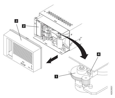
Figure 196. Model C00 Drive Inner Cover Configuration
