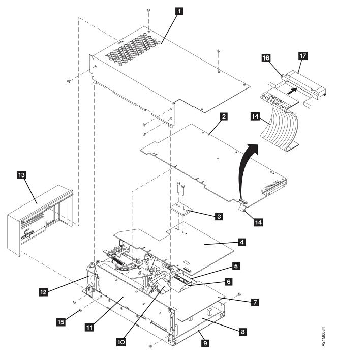
Figure 274. Base Drive FRU Breakout
