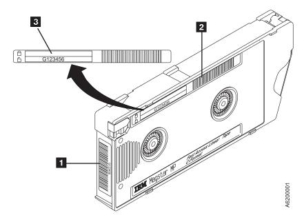
Figure 255. Label Placement on 3570 Cartridge
