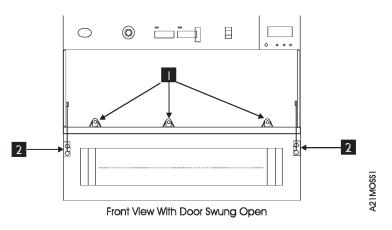
Figure 336. Library Front Door Assembly—Front View Holding Screws
