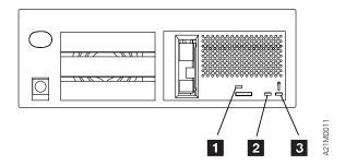
Figure 301. Drive Indicators for Drive-Only Models
