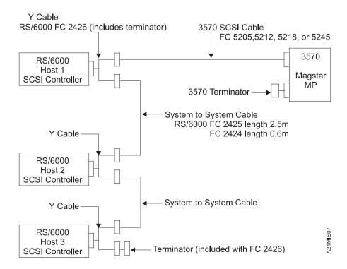
Figure 236. Multiple RS/6000 Systems Attached to a 3570
