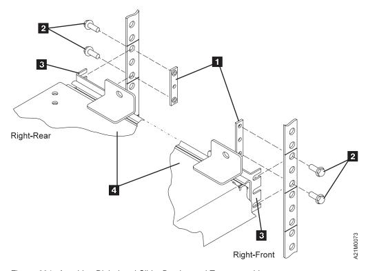
Figure 204. Attaching Right-hand Slide, Bracket and Tray assembly
