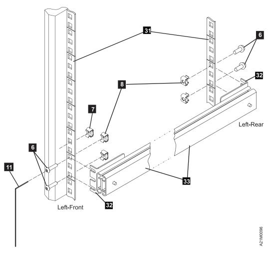
Figure 213. Attaching Left-hand Slide and Bracket assembly
