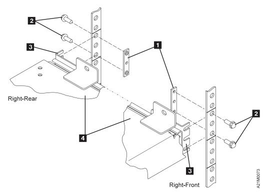
Figure 188. Support Slide, right side, Models C11 and C12
