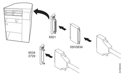
Figure 223. Installing the SCSI System Cable at the AS/400 Host (Initiator)
