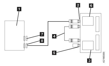
Figure 232. AS/400 FC 6501—Split Configuration (single host, one IOP, one port)
