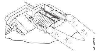
Figure 322. Thin-film cable installation
