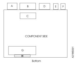
Figure 276. Library Control Card Cable and Bar Code Reader Card Layout
