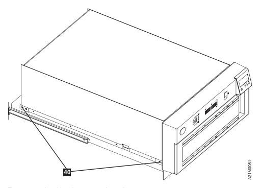
Figure 190. Attaching the 3570 to the rack tray.
