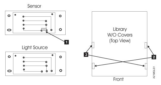
Figure 277. Library Global Sensor Component Identification and Locations
