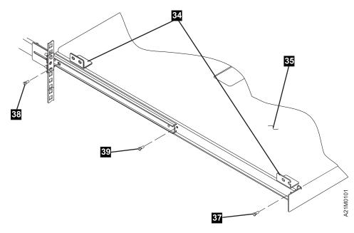
Figure 215. Attaching Tray to Left-hand Slide
