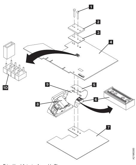
Figure 318. Base Drive Head-Actuator Assembly Close-up
