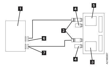
Figure 233. AS/400 FC 6501—Split Configuration (single host, one IOP, both ports)
