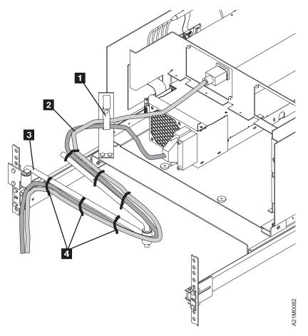
Figure 237. Cable Routing, Model C11
