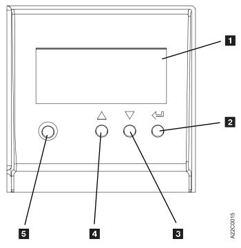
Figure 55. Operator Panel Display for Library Models
