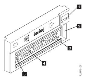
Figure 50. Magazine and Cartridge Locations, Models C21 and C22
