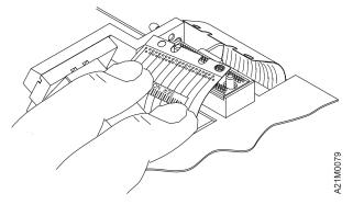
Figure 321. Thin-film cable installation
