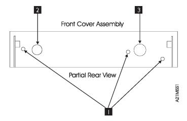
Figure 335. Library Front Door Assembly—Rear View Holding Screws
