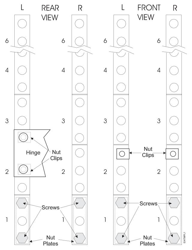
Figure 202. EIA Rack Template for Models C11 and C12
