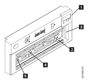
Figure 38. Magazine and Cartridge Locations, Models C21 and C22
