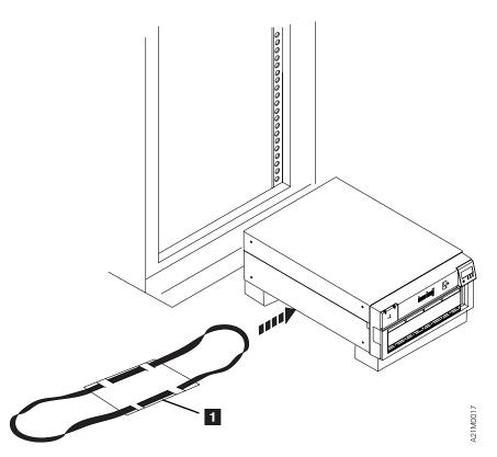
Figure 208. Sliding Strap Under Drive
