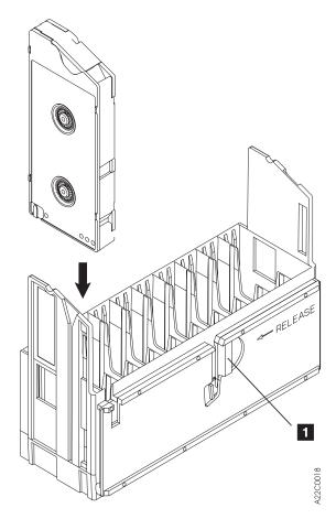
Figure 251. Loading a Cartridge in a Magazine (with Operator Side Facing Down)
