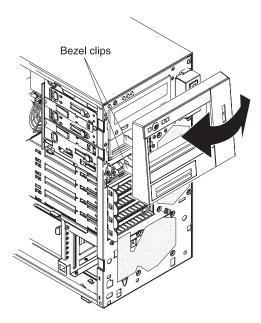
Figure 3. Removing the upper bezel
