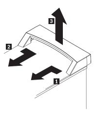
Figure 5. Removing the top handle
