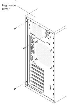
Figure 7. Removing the right-side cover
