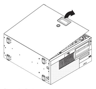
Figure 13. Installing the top cover
