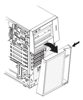
Figure 2. Removing the lower bezel
