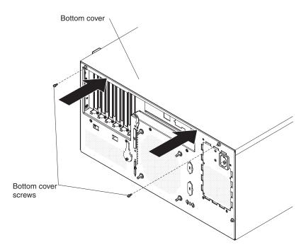
Figure 10. Installing the new bottom cover
