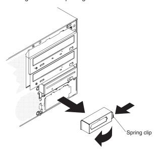
Figure 8. Removing the front USB housing
