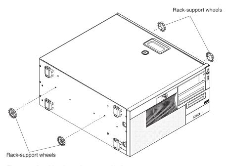
Figure 15. Attaching the rack-support wheels
