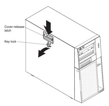
Figure 1. Removing the left-side cover
