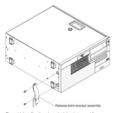
Figure 14. Installing the release-latch-bracket assemblies
