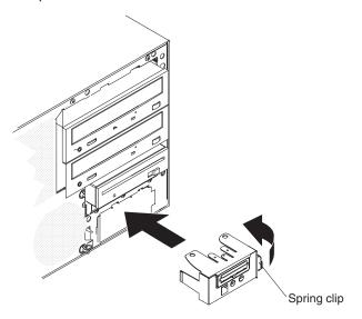
Figure 11. Reconnect the front USB housing
