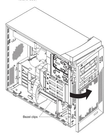
Figure 4. Removing the one-piece bezel
