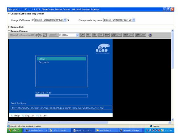
Figure 26: SUSE GRUB Screenshot of a Successful iSCSI boot
