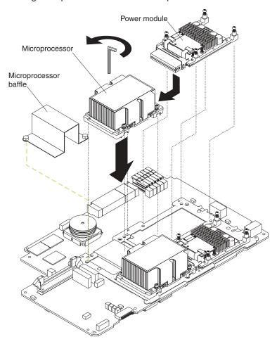
c. Ensure that the socket lock is in the fully open (unlocked) position to permit plugging in the microprocessor. Use the hex wrench provided with the
