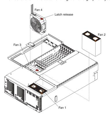
Each fan has an LED to help you detect a problem. When the fan is operating correctly, this LED is off. If a fan stops working, the Light Path Diagnostics feature will light the System-error LED on the front of the server, indicating that there is a problem and guide you to the defective fan. When this occurs, first identify the defective fan; then, using the appropriate procedure, remove and replace the fan.
