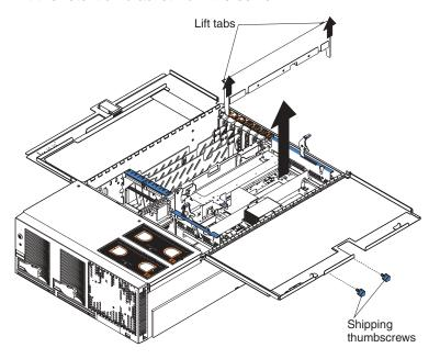
6. Remove the processor-board assembly from the server:
