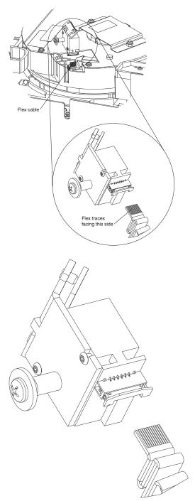
9. Tighten the strain relief mechanism on the ZIF connector.
