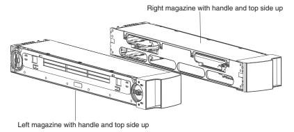
6. Install the two screws to attach the handle securely to the magazine.
