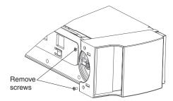
2. Unsnap the handle carefully, ensuring you do not break the hinge.
