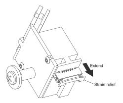
8. Seat the end of the flex cable into the ZIF connector as far as it will go.
