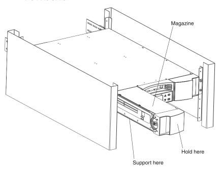
3. The magazine is correctly installed when you feel it click into place and the front is flush with the front panel.
