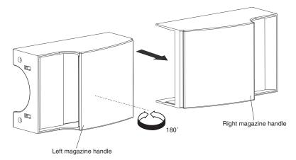
4. Rotate the magazine 180 degrees so that what was the front of the magazine is now the back.
