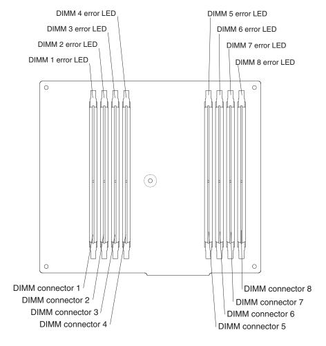
b. The following illustration shows the internal connectors and LEDs on the 16-DIMM-connector memory board in the memory cassette.
