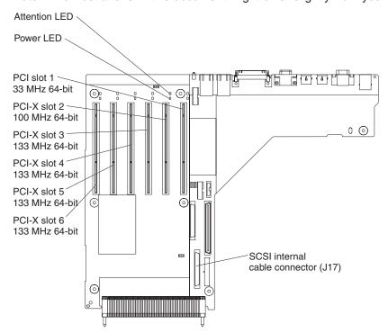
• Each PCI/PCI-X slot is on a separate PCI bus.
