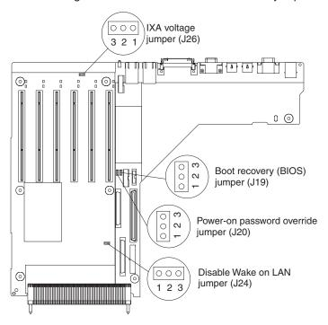
The I/O board contains three-pin jumper blocks. The following table describes the purposes of the jumpers.
