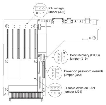
3. Locate the power-on password override jumper (J20), removing any components that impede access to the jumper.
