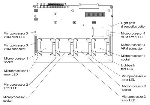
5. Press and hold down the light-path diagnostics button on the microprocessor board. The LEDs will be lit while the button is pressed. You can light the LEDs for a maximum of 2 minutes, after which power is no longer available for the LEDs.
