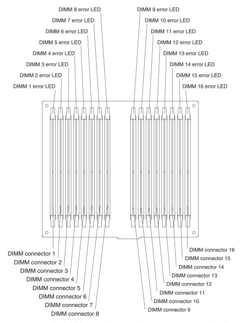
4. If necessary, open the DIMM access doors on the memory cassette to view the DIMM LEDs.
