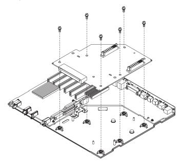
16. Set the assembly on a firm and static-protective work surface; then, remove the six screws that secure the power backplane to the backerplate and set the screws in a safe place.
