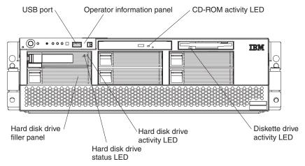
**USB port:** You can connect a USB device to this connector.
