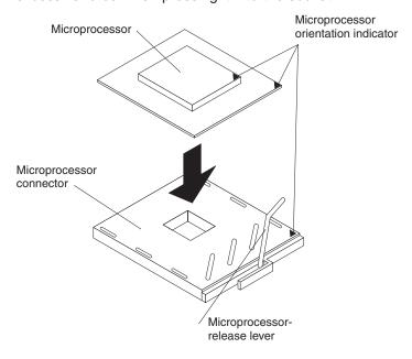
11. Close the microprocessor-release lever to secure the microprocessor.
