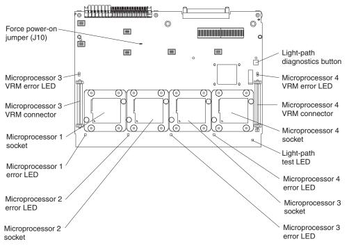
The microprocessor board contains the force power-on jumper (J10), a three-pin jumper block. The default position is pins 1 and 2. Move the jumper to pins 2 and 3 to force the server to start up when you connect the server to ac power.
