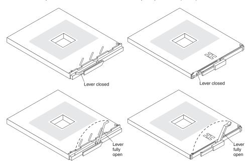
**Attention:** You must ensure that the locking lever on the microprocessor socket is in the fully-open position before you insert the microprocessor in the socket. Failure to do so might result in permanent damage to the microprocessor, microprocessor socket, and microprocessor-tray assembly.
