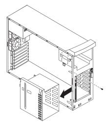
To replace the hard disk drive cage, reverse the steps.
