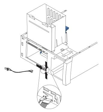
9. Note where the power-switch and LED panel cables connect to the system board; then, carefully disconnect the cables from the system board.
