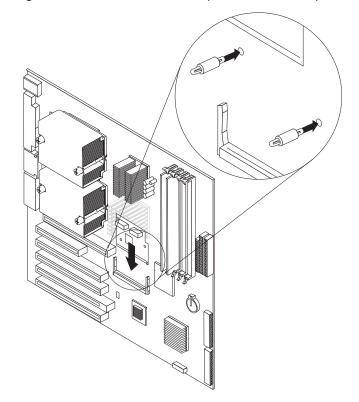
**Note:** If there is a gap between the adapter and the retaining clips, the adapter has not been properly installed. In this case, open the retaining clips and remove the adapter; then, reinsert the adapter. You might need to disengage the locking clips on the two stand-offs to remove the adapter.
