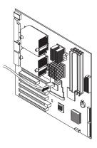
9. Using a pair of pliers, squeeze the stand-off pins and pull the mini-PCI card up and out of the slot.
