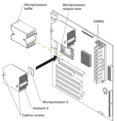
Complete the following steps to install an additional microprocessor:
