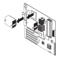
6. To install a microprocessor, see "Installing an additional microprocessor" on page 57
