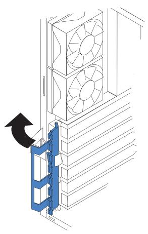
To replace the rear adapter retainer, reverse the steps.
