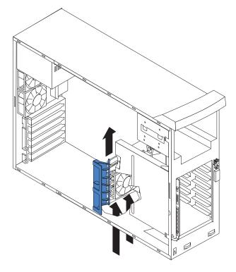
7. Use side cutters to cut the four rubber extensions on the adapter-support bracket.
