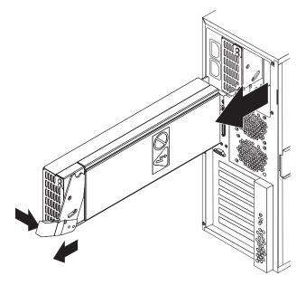
3. Make sure the power-supply handle is in the open position; then, slide the power supply all the way into the chassis before placing the power-supply handle into the locked position.
