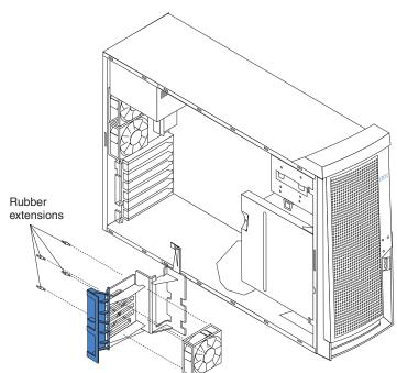
8. Gently pry the fan away from the adapter-support bracket and lift it up and out.
