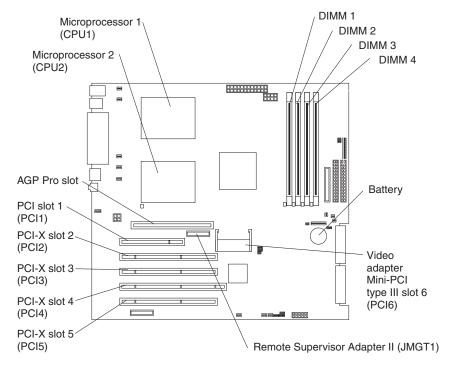
The following illustration shows the system-board connectors for user-installable options.
