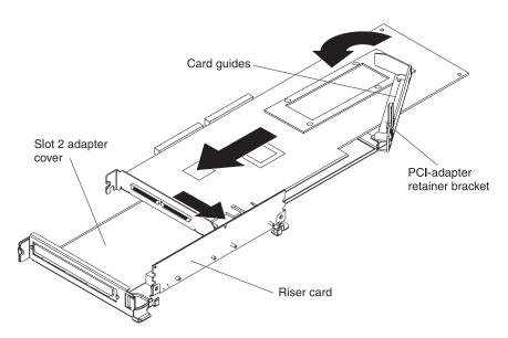
Figure 22. Riser card and adapter cover removal
