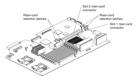
Figure 19. Adapter connectors and latches
