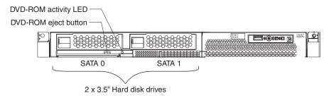
Figure 4. Server with 3.5-inch SATA simple swap hard disk drive configuration
