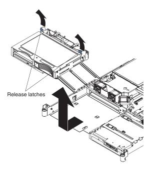
Figure 60. Drive tray assembly removal
