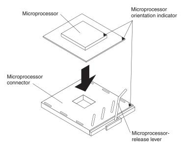
Figure 37. Microprocessor installation
