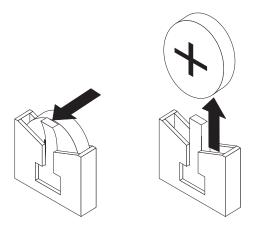
Figure 46. Battery removal
