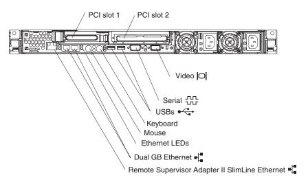
Figure 50. Cable identifiers, rear view of server
