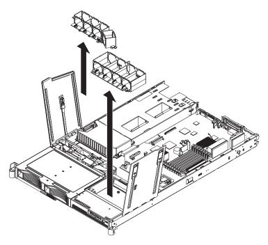
Figure 59. Fan bracket removal
