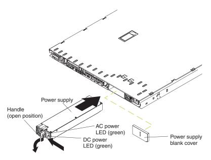
Figure 42. Power supply installation
