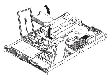
Figure 61. Power backplane removal
