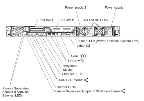
Figure 47. Cable identifiers, rear view of server
