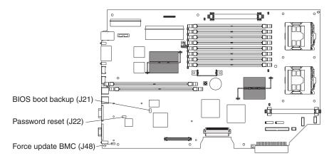
Figure 14. BIOS boot backup jumper location
