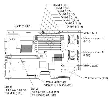
Figure 62. System-board option connectors
