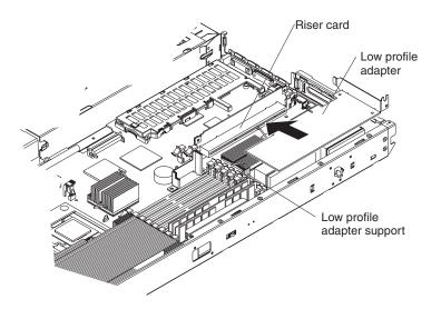
Figure 20. Low-profile adapter installation, slot 1
