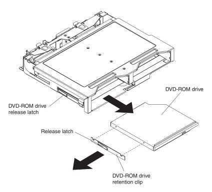
Figure 30. Removing an internal DVD-ROM drive
