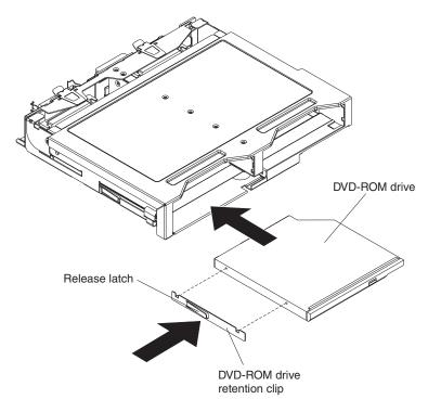
Figure 32. Installing an internal DVD-ROM drive
