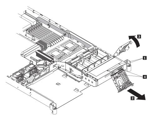
Figure 58. Operator information panel removal
