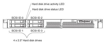
Figure 2. Server with a 2.5-inch SCSI hot-swap hard disk drive configuration
