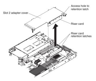
Figure 21. Slot 2 connectors and latches
