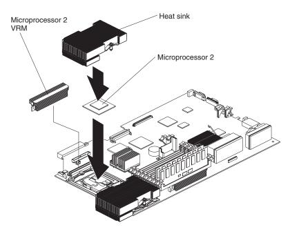
Figure 38. Heat sink installation
