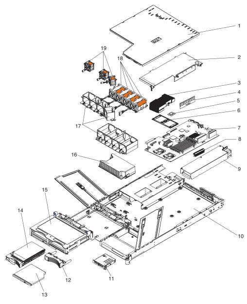
Figure 67. Parts, Type 1879 and Type 8837
