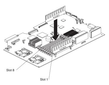
Figure 33. Memory module installation
