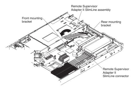
Figure 25. Installing the Remote Supervisor Adapter II SlimLine
