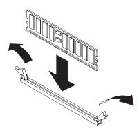
Figure 34. DIMM retainer clips
