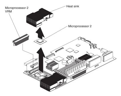
Figure 57. Microprocessor removal
