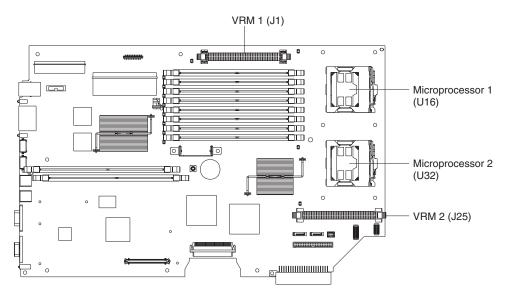
Figure 35. Location of microprocessor and VRM sockets
