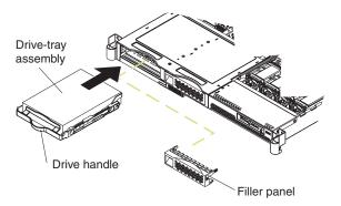
Figure 28. Installing a simple-swap hard disk drive
