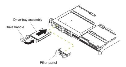
Figure 26. 2.5-inch hot-swap hard disk drive installation
