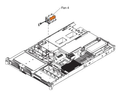
Figure 39. Installing fan 4 after installing a second microprocessor
