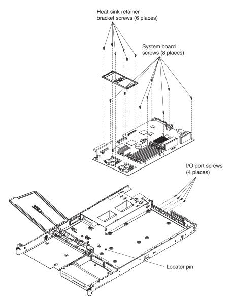
Figure 66. System board removal
