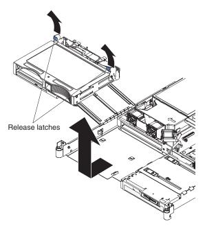
Figure 29. Removing the hard drive cage
