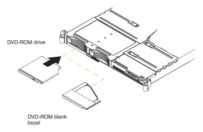
Figure 31. Internal DVD-ROM drive and blank bezel
