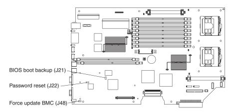
Figure 15. Password reset jumper location
