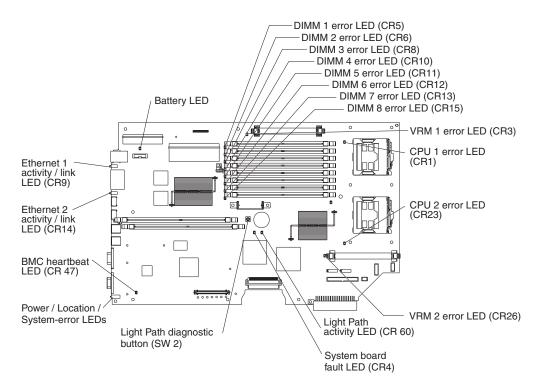
Figure 8. System-board LEDs
