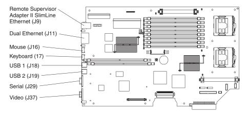
Figure 64. System-board external connectors
