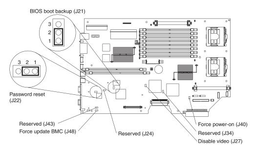
Figure 65. System-board jumpers
