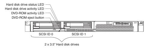
Figure 3. Server with a 3.5-inch SCSI hot-swap hard disk drive configuration
