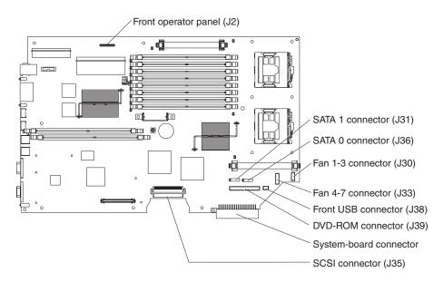
Figure 63. System-board internal connectors
