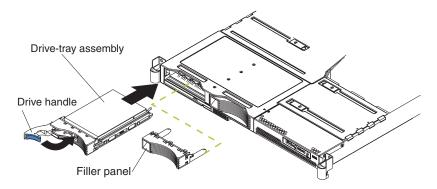
Figure 27. 3.5-inch hot-swap hard disk drive installation
