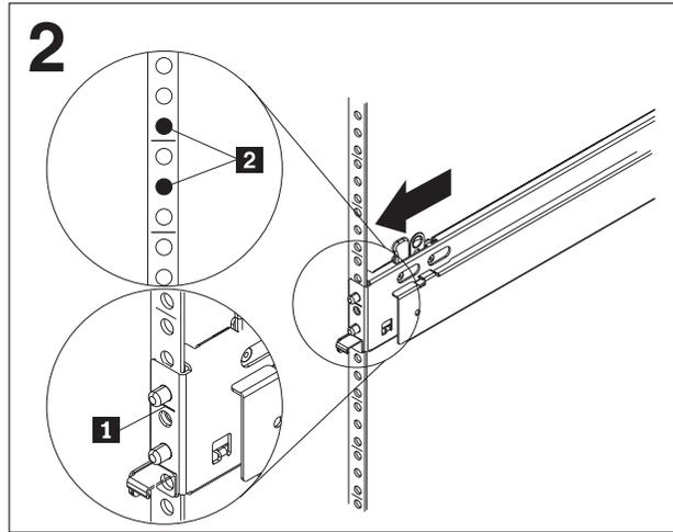
Push outward on the slide-rail latch **1**; then, pull the latch **2** back to open the slide rail. The latch catches to stay open. Open the other end of the slide rail; then, do the same for the other slide rail. **Note:** If you are installing the server in the top of the rack or directly under another server or device, install the cable-management-arm bracket on the slide rail. Go to step 6 to install the cable-management-arm bracket; then, continue with step 2.
