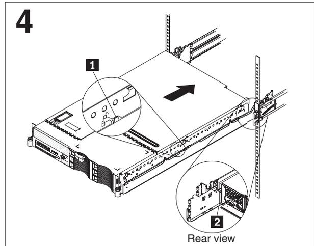
Carefully slide the server along the slide rails approximately 1 inch toward the rack to lock the server on the slide rails.
