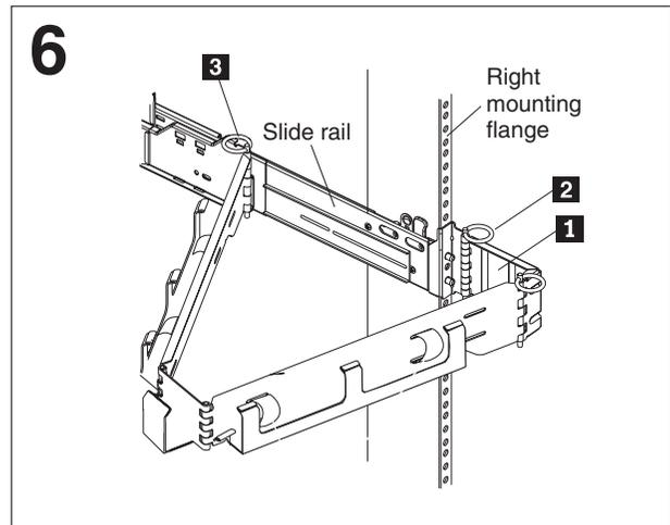
Attach the cable-management-arm bracket **1** to the cable-management assembly and then to the rear of the slide rail, using the hinge pins **2**. Attach the free end of the cable-management assembly to the slide rail, using a hinge pin **3**.
