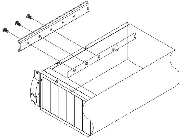
4. Attach the adjustable rear-rack rails to the front-rack rails. (The four 10-32 x 1/2-inch screws and nuts are provided in the miscellaneous hardware bag.)
