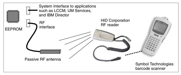
Figure 2. Asset ID EEPROM and passive antenna
