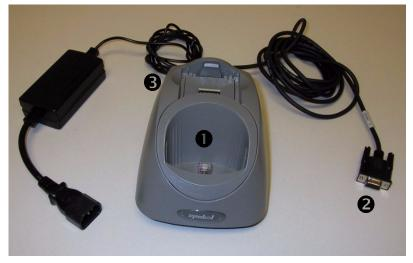
Figure 4. Recharger and host connection cradle
