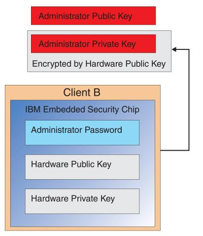
Figure 13. The Administrator private key is encrypted with the Client B hardware key.
