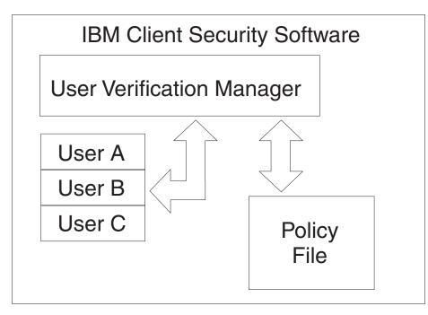
Figure 21. User Verification Manager controls each user's credentials and enforces security policies.
