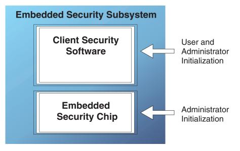
Figure 1. IBM Embedded Security Subsystem components
